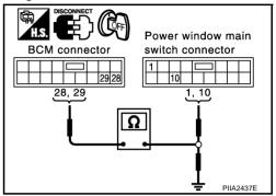
4. Check continuity between BCM connector M1 terminal 28, power window sub-switch connector D43 terminal 10, and between BCM connector M1 terminal 28 and ground.
