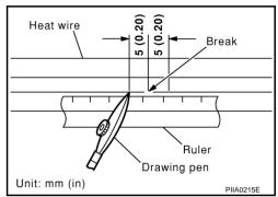
After repair has been completed, check repaired wire for continuity. This check should be conducted 10 minutes after silver composition is deposited.
