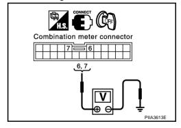
Door switch Combination meter connector
