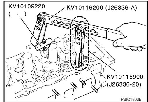
4. Remove valve spring retainer and valve spring.
