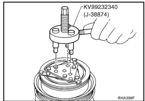
2. Remove clutch disc using clutch disc puller.
