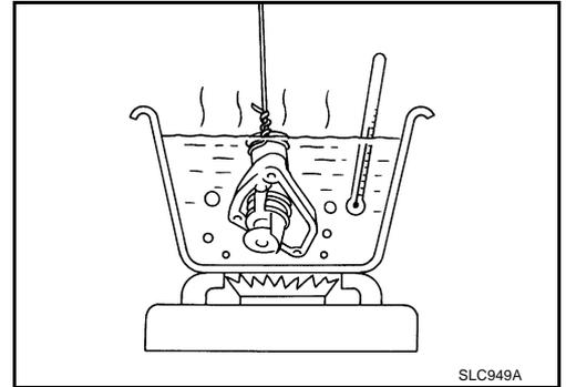
3. Check if valve is closed at 5°C (9°F) below valve opening temperature.
