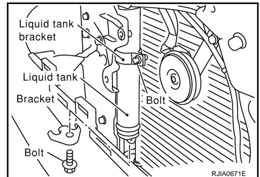
6. Lift liquid tank upwards. Remove bracket from protruding part of condenser.
