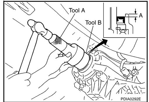
2. Align the matchmark of mainshaft with the mark of companion flange, then install the companion flange.
