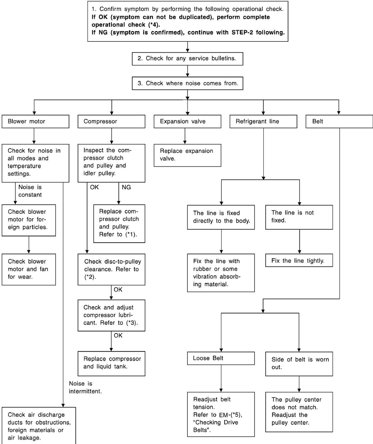
\*1 Compressor clutch, [ATC-142. "REMOVAL"](#) .
