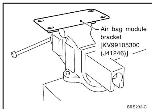
3. Match the hole in air bag module bracket (held in vise) and front passenger air bag module and fix them with one bolt [M8 × 25 - 30 mm (0.98 - 1.18 in)].
