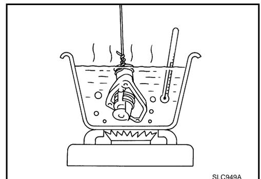
3. Then check if valve closes at 5°C (9°F) below valve opening temperature.
