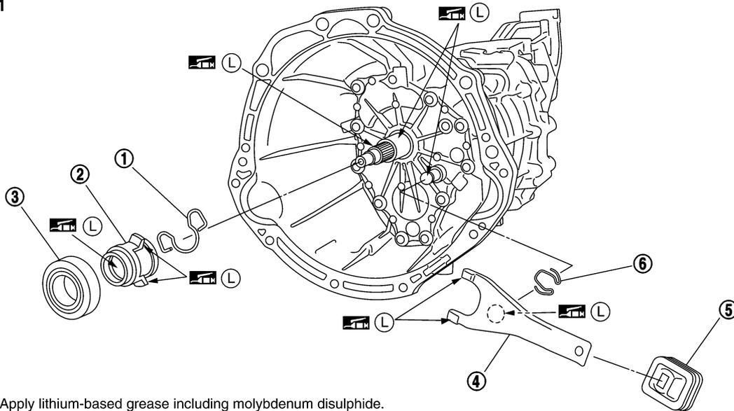
(L) : Apply lithium-based grease including molybdenum disulphide.
