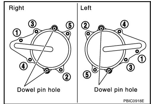
14. Install oil pans (upper and lower). Refer to [EM-30, "OIL PAN AND OIL STRAINER"](#) .
