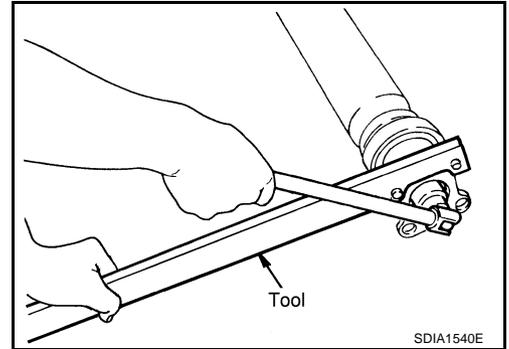
5. Remove center bearing with tool and press.
