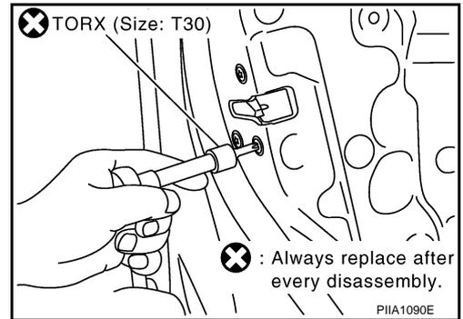
8. Remove the exterior handle mounting bolts, move the outside handle assembly backward, and then remove it from the panel in front of the outside handle escutcheon.
