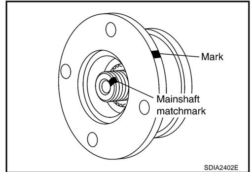
3. Using flange wrench, install the self-lock nut of companion flange and tighten to the specified torque. Refer to [TF-52, "COMPONENTS"](#).
