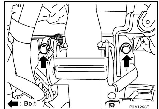
2. Remove bolts and screws, and remove instrument panel and pad from passenger door opening portion.
