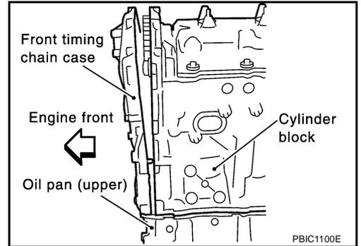
ii. Since front timing chain case is offset for difference of bolt holes, tight bolts temporarily with holding front timing chain case from front and top as shown in the figure.
