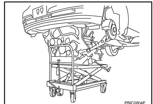
2. Remove rear engine mounting member bolts.
