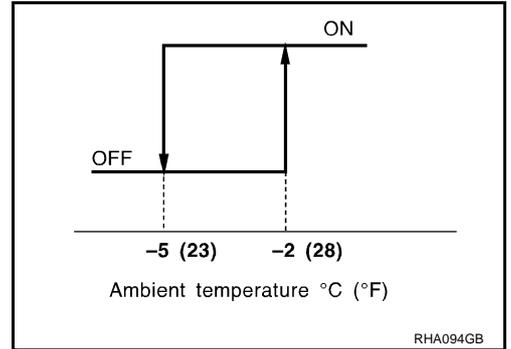
When intake air temperatures are higher than  $1^{\circ}\text{C}$  ( $34^{\circ}\text{F}$ ), the compressor turns ON. The compressor turns OFF when intake air temperatures are lower than  $-5^{\circ}\text{C}$  ( $23^{\circ}\text{F}$ ).
