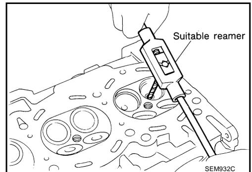
4. Heat cylinder head to 110 to 130°C (230 to 266°F) by soaking in heated oil.
