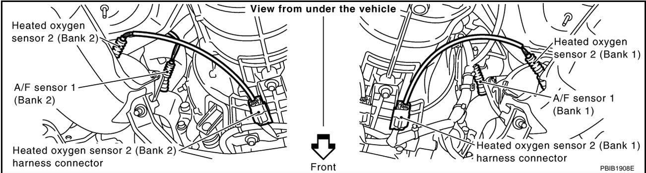
4. Check harness continuity between HO2S2 terminal 4 and ECM terminal 78. Refer to Wiring Diagram.
