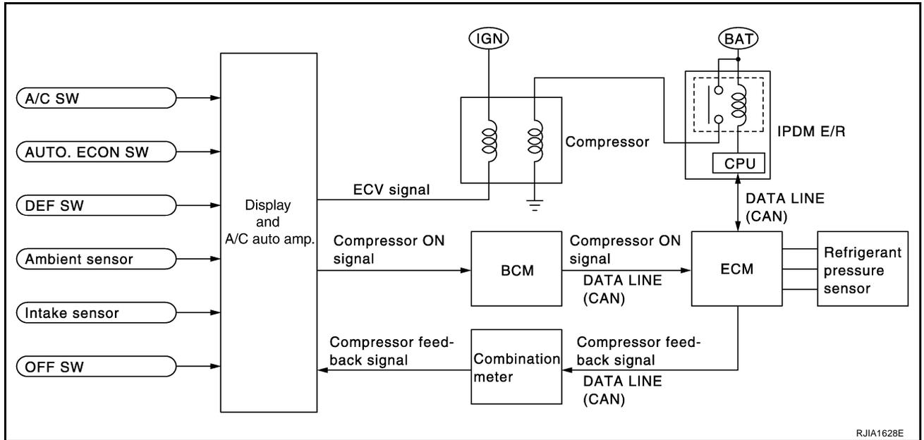
When A/C switch, AUTO.ECON switch or DEF switch is pressed, display and A/C auto amp. inputs compressor ON signal to BCM.
