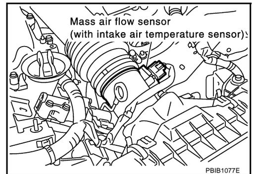
3. Check voltage between mass air flow sensor terminal 5 and ground.
