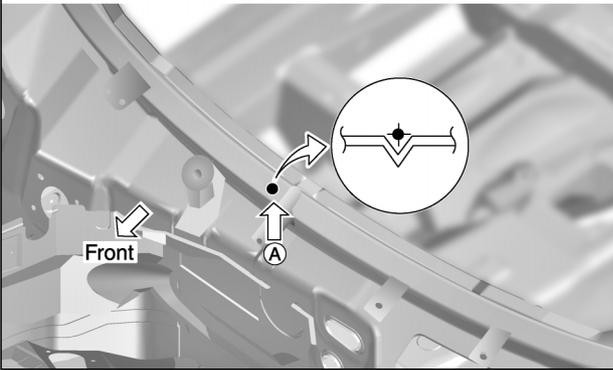
(B) : Front roof flange end of center positioning mark
