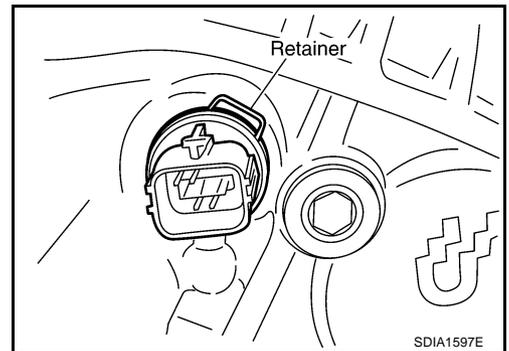
9. Set temperature sensor and tighten bolt to the specified torque. Refer to [TF-52, "COMPONENTS"](#).
