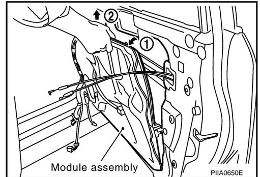
8. Disconnect the harness connector for the module assembly, and unclip the harness from the back.
