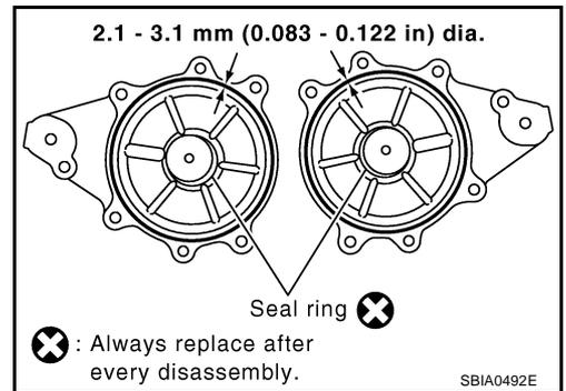
c. Install collared O-ring in front timing chain case oil hole (left and right sides).
