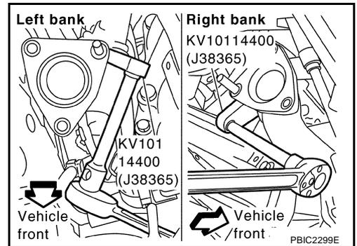
9. Remove water pipe and heater pipe on both right and left side. Refer to [CO-29, "WATER OUTLET AND WATER PIPING"](#).
