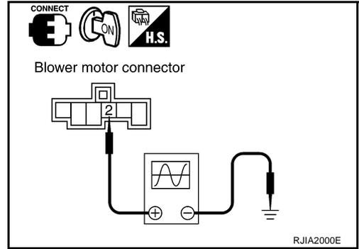
3. Vary the fan speed between Lo and Hi and confirm the duty ratios between blower motor harness connector M62 terminal 2 (G) and ground using an oscilloscope. Usual terminal 2 (G) drive signal duty ratios are shown in the table below.
