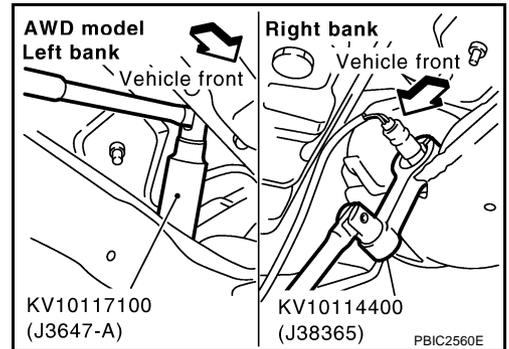
6. Remove exhaust mounting bracket between three way catalyst (right and left bank) and transmission. Refer to [EX-3, "EXHAUST SYSTEM"](#).
