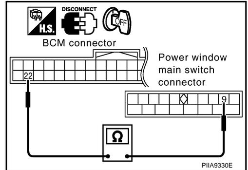
4. Check continuity between BCM connector M1 terminal 22 and front power window sub-switch (front passenger side) (door lock and unlock switch) connector D36 terminal 11.
