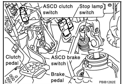
2. Check voltage between stop lamp switch terminal 1 and ground with CONSULT-II or tester.
