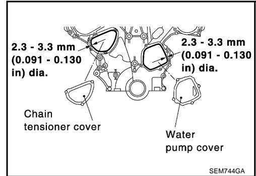
12. Install front timing chain case as follows:
