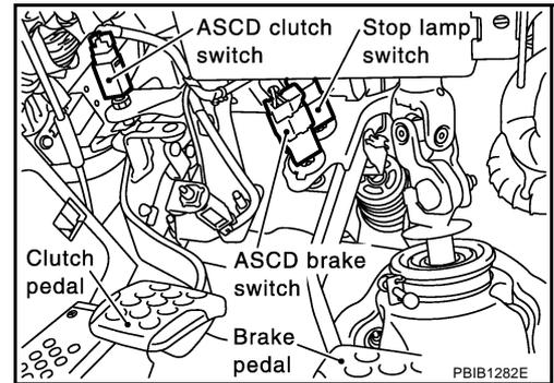
4. Check voltage between ASCD clutch switch terminal 1 and ground under the following conditions with CONSULT-II or tester.
