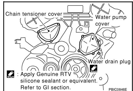
8. Remove chain tensioner cover and water pump cover from front timing chain case.
