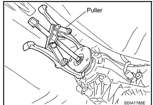
5. Remove the rear oil seal using a puller.
