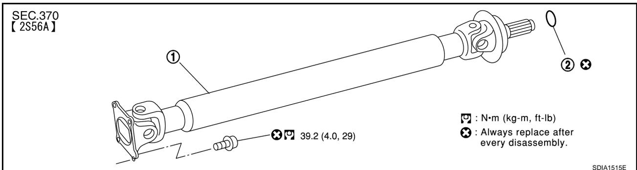
1. Propeller shaft assembly
