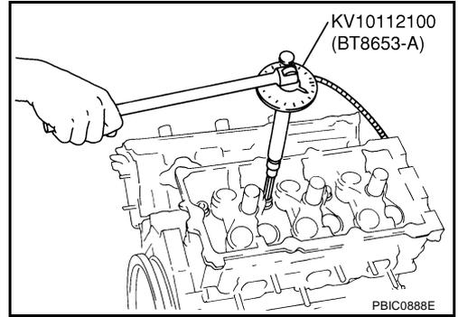
4. After installing cylinder head, measure the distance between front end faces of cylinder block and cylinder head (left and right banks).
