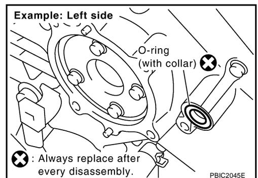
d. Being careful not to move seal ring from the installation groove, align dowel pins on front timing chain case with holes to install intake valve timing control covers.
