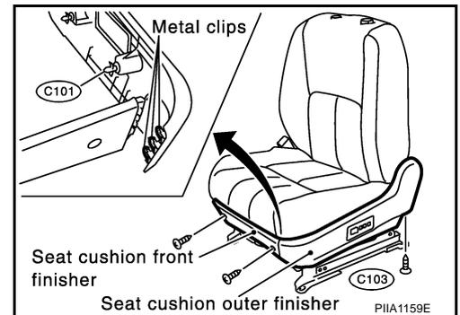
2. Remove the power seat switch assembly.
