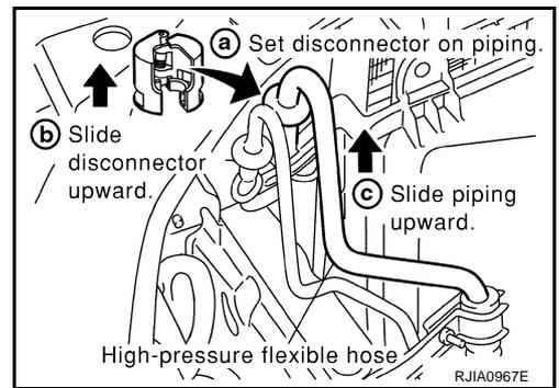
5. Remove mounting nut for high-pressure flexible hose, and then remove high-pressure flexible hose.
