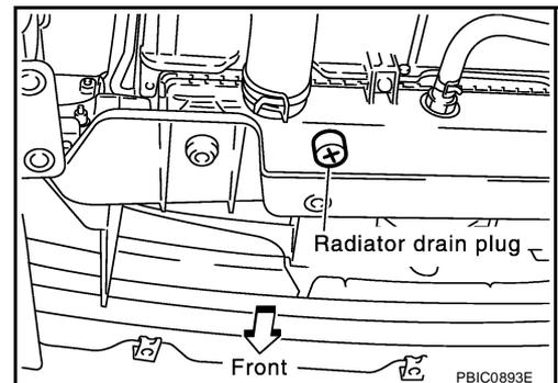
When drain all of engine coolant in the system, open drain plugs on engine cylinder block. Refer to [EM-122, "DISASSEMBLY"](#) .
