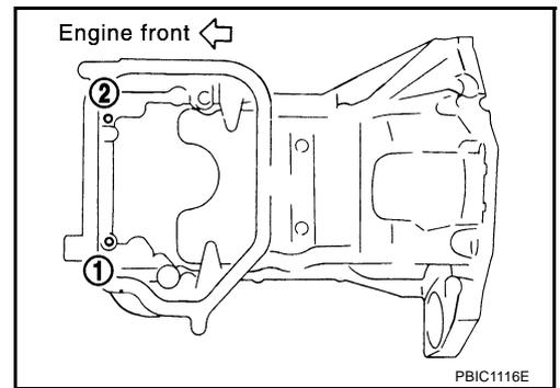
7. Install oil pan (lower). Refer to [EM-30, "OIL PAN AND OIL STRAINER"](#).
