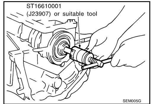
13. Remove rear oil seal retainer.
