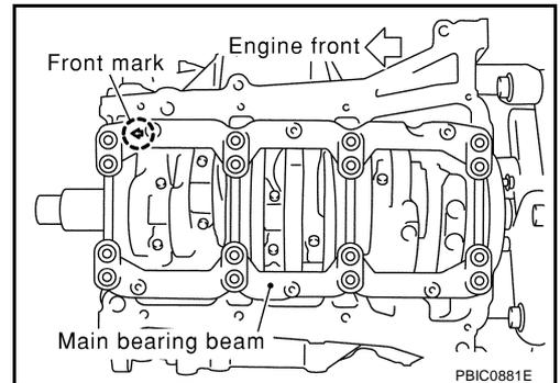
9. Inspect outer diameter of main bearing cap bolt. Refer to [EM-147, "MAIN BEARING CAP BOLT OUTER DIAMETER"](#).
