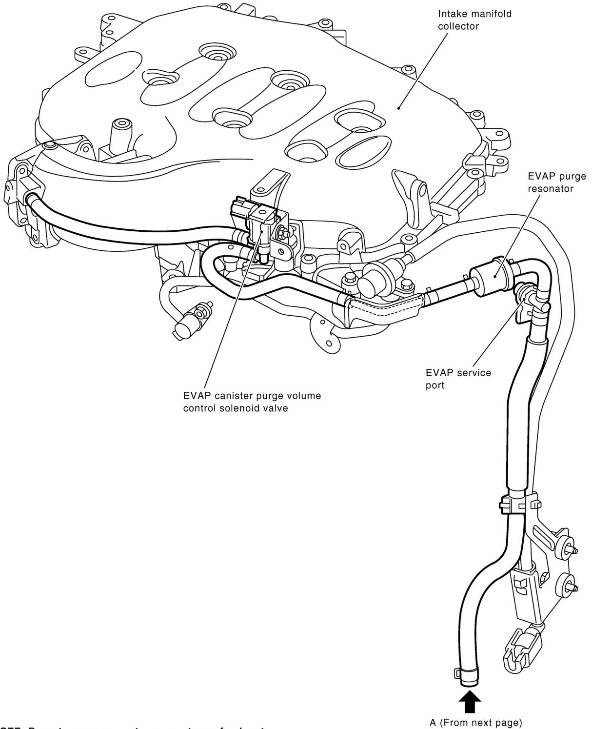
**NOTE: Do not use soapy water or any type of solvent while installing vacuum hose or purge hoses.**
