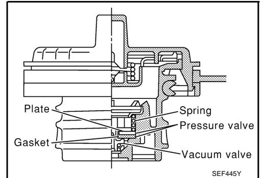
2. Check valve opening pressure and vacuum.
