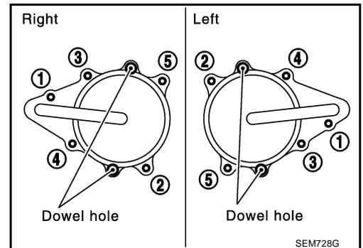
11. Remove collared O-ring from front timing chain case (left and right side).
