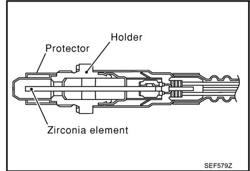
An electronic circuit controls the pump current through the oxygen-pump cell so that the composition of the exhaust gas in the diffusion gap remains constant at  $\lambda = 1$ . Therefore, the A/F sensor 1 is able to indicate air/fuel ratio by this pumping of current. In addition, a heater is integrated in the sensor to ensure the required operating temperature of 700 - 800°C (1,292 - 1,472°F).
