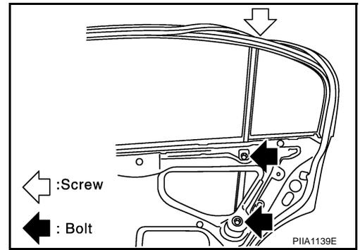
8. Remove the glass mounting bolts, and remove the door glass.
