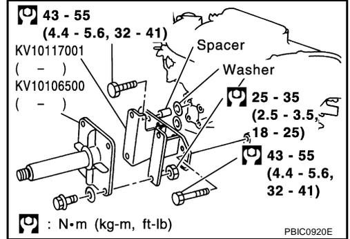
5. Lift engine, and mount it onto engine stand (SST).
