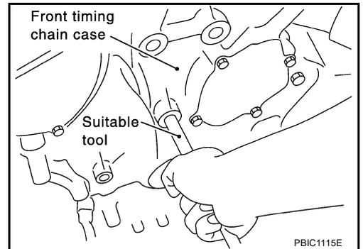
e. Tighten bolts to the specified torque in numerical order as shown in the figure.
