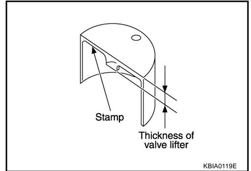
Available thickness of valve lifter: 27 sizes with range 7.88 to 8.40 mm (0.3102 to 0.3307 in) in steps of 0.02 mm (0.0008 in) (when manufactured at factory). Refer to [EM-153, "Available Valve Lifter"](#) .
