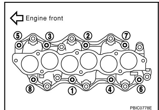
5. Remove intake manifold gaskets.
