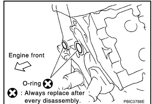
32. Remove timing chain tensioners (secondary) from cylinder head as follows, if necessary.
