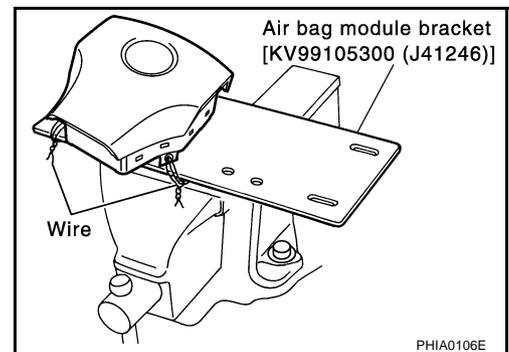
4. Connect deployment tool adapter (SST: J38381-80) to air bag module connector and deployment tool connector [SST: KV99106400 (J38381)].
