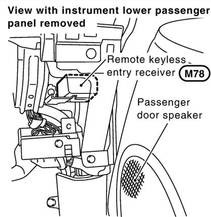
View with instrument lower passenger panel removed
