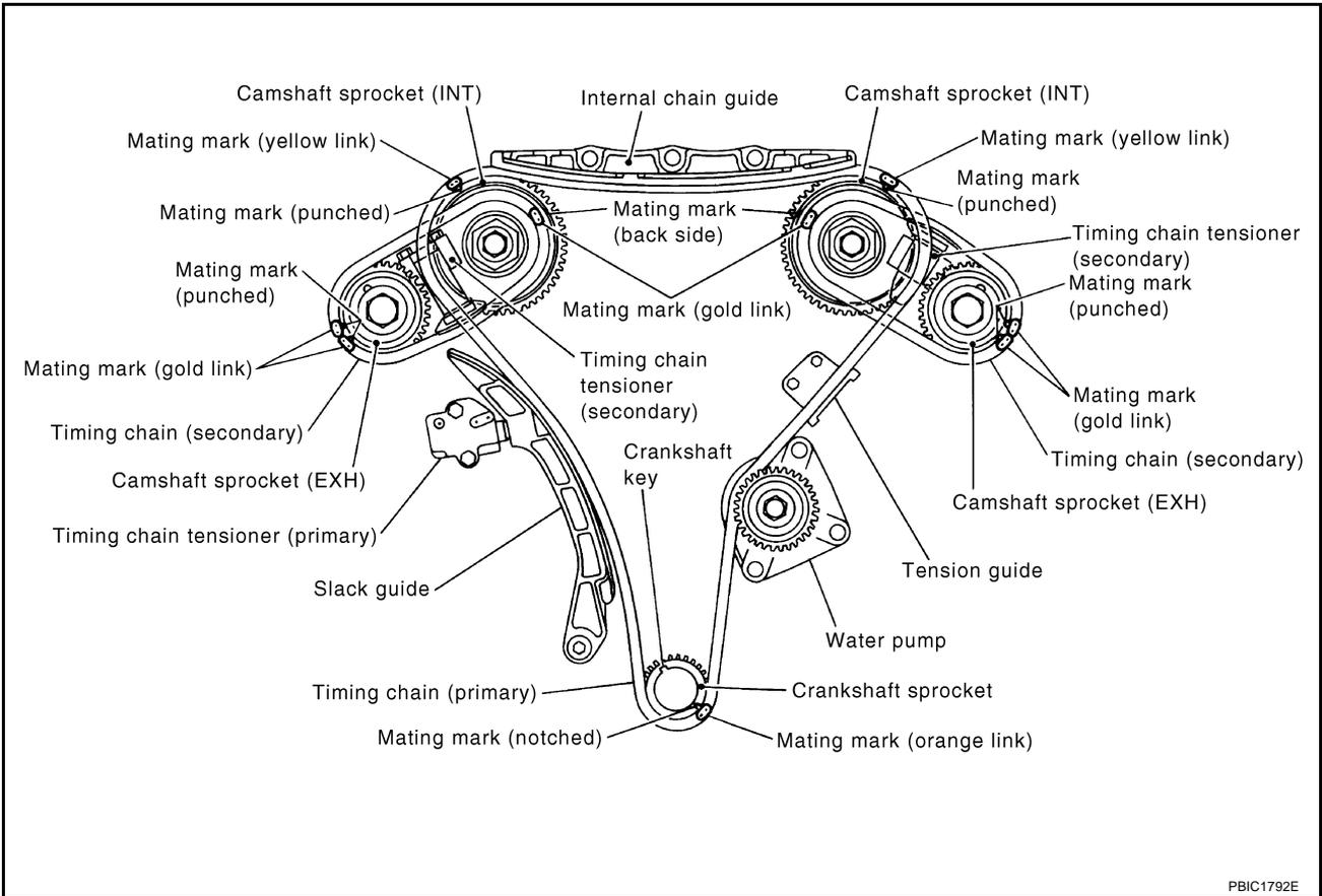
1. Install timing chain tensioners (secondary) to cylinder head as follows if removed. Refer to [EM-89, "INSTALLATION"](#).
