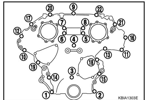
f. After all bolts tightened, retighten them to the specified torque in numerical order as shown in the figure.
