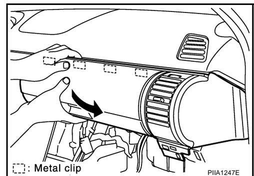
3. After removing, remove side ventilator grille and lid. Refer to [IP-19, "CENTER BOX ASSEMBLY"](#) .
