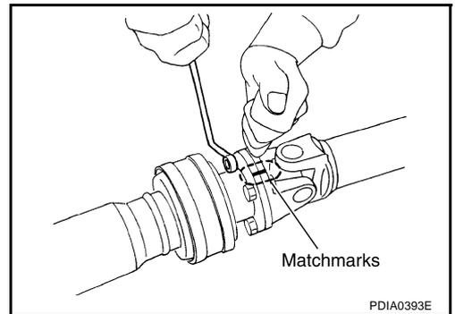
2. Put matchmarks onto the center flange and propeller shaft end as shown.
