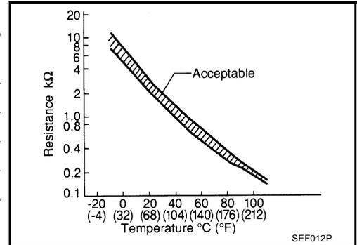
\*: This data is reference value and is measured between ECM terminal 73 (Engine coolant temperature sensor) and ground.
