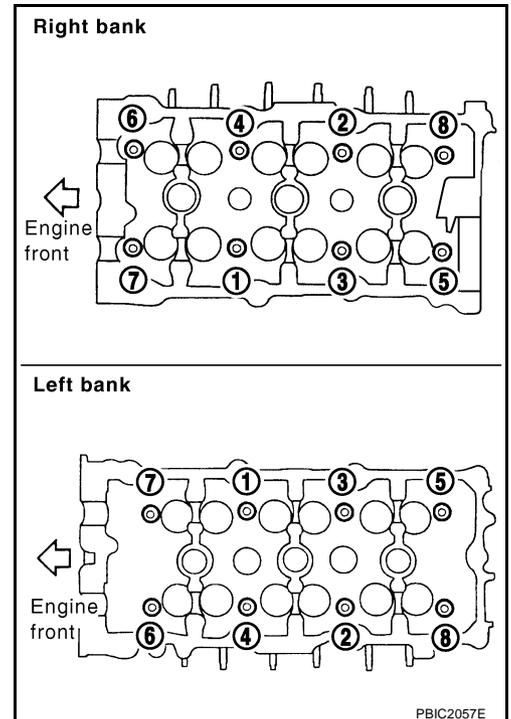
6. Remove cylinder head gaskets.
