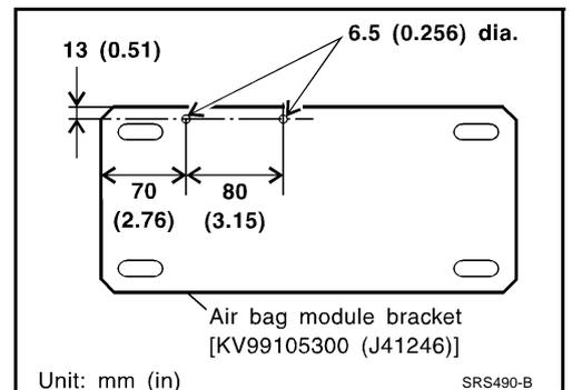
2. Firmly secure air bag module bracket [SST: KV99105300 (J41246)] in a vise.
