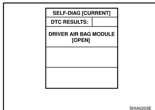
If no malfunction is detected on “SELF-DIAG [CURRENT]” even though malfunction is detected in “SRS Operation Check”, check the battery voltage. If the battery voltage is less than 9 V, charge or replace the battery. Then go to [SRS-24. "DIAGNOSTIC PROCEDURE 3"](#) . If the battery voltage is OK, go to [SRS-26. "DIAGNOSTIC PROCEDURE 4 \(CONTINUED FROM DIAGNOSTIC PROCEDURE 2\)"](#) to diagnose the following cases:
