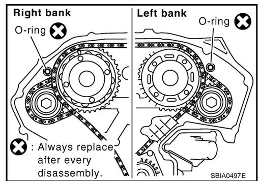
d. Assemble front timing chain case as follows:
