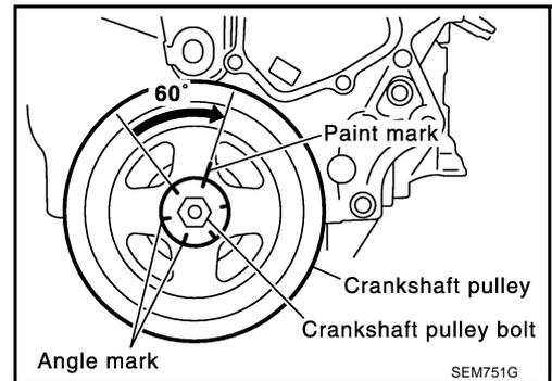
17. Rotate crankshaft pulley in normal direction (clockwise when viewed from engine front) to confirm it turns smoothly.
