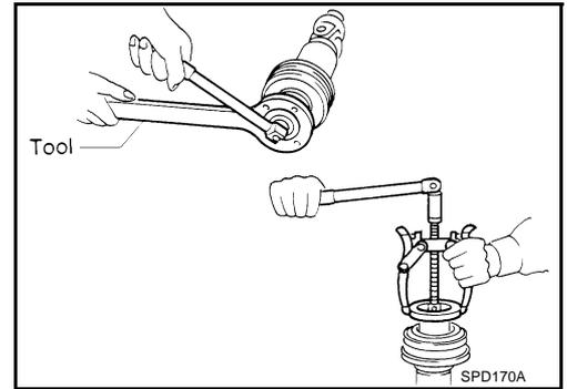
6. Remove center bearing with tool and press.
