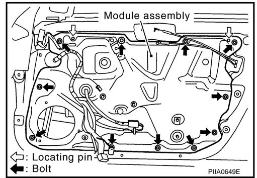
7. Draw out the locating pins on the upper of the module assembly from the door panel, and then remove the module assembly by drawing forward and moving upward.
