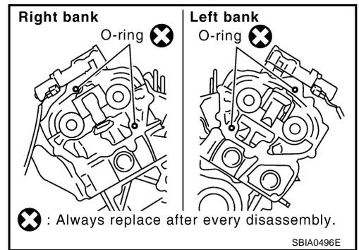
31. Remove O-rings from cylinder block.
