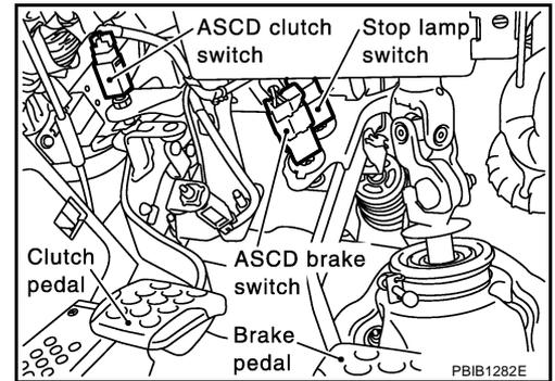
4. Check voltage between ASCD clutch switch terminal 1 and ground under the following conditions with CONSULT-II or tester.
