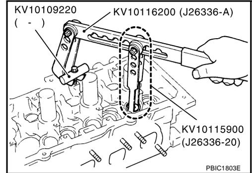
5. Remove valve spring retainer and valve spring.
