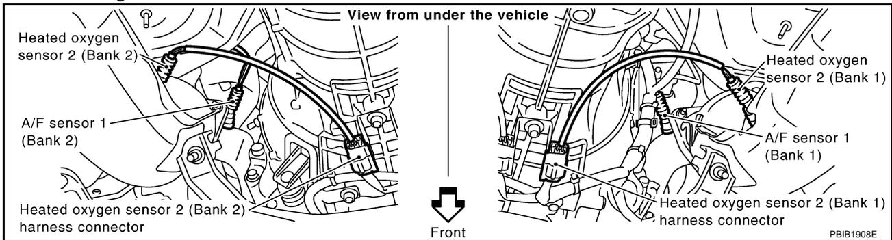
**Tightening torque: 40 - 60 N-m (4.1 - 6.1 kg-m, 30 - 44 ft-lb)**
