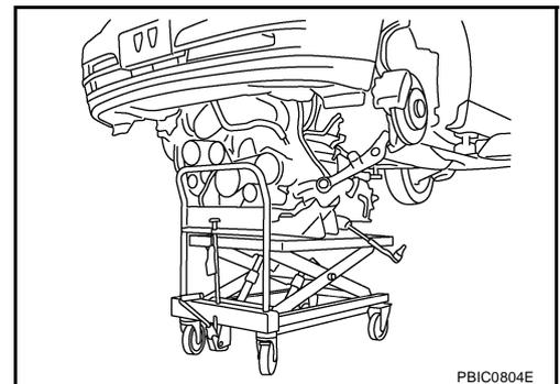
2. Remove rear engine mounting member bolt.
