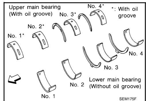
6. Install crankshaft to cylinder block.
