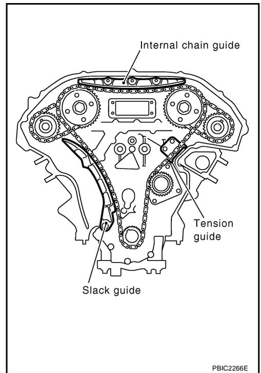
27. Remove timing chain (primary) and crankshaft sprocket.
