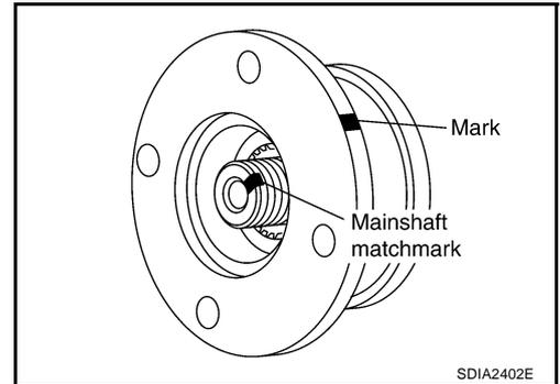
22. Tighten self-lock nut to the specified torque, with flange wrench. Refer to [TF-52, "COMPONENTS"](#).
