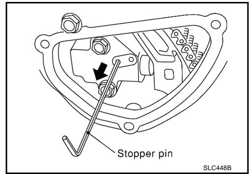
4. Install chain tensioner cover and water pump cover as follows:
