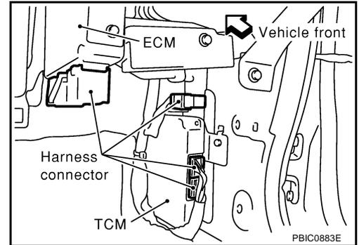
2. Disconnect engine room harness connectors at unit side TCM (A/T models), ECM and other.
