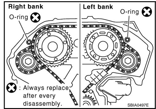
23. Remove water pump cover and chain tensioner cover from front timing chain case.
