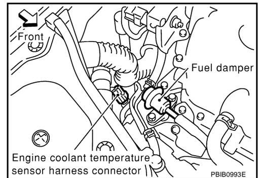
3. Check voltage between ECT sensor terminal 1 and ground with CONSULT-II or tester.
