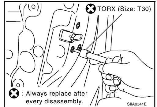
5. Remove the outside handle mounting bolts, and move the handle backward to disengage it from the panel in front of the outside handle escutcheon, then remove the handle.
