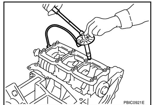
11. Inspect outer diameter of connecting rod bolt. Refer to [EM-148, "CONNECTING ROD BOLT OUTER DIAMETER"](#).
