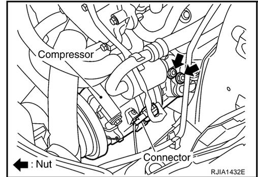
7. Disconnect compressor (ECV) connector.
