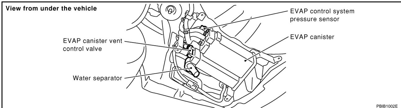
2. Check sensor harness connector for water.
