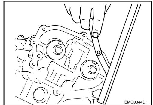
7. Check and adjust valve clearance. Refer to [EM-91, "Valve Clearance"](#).
