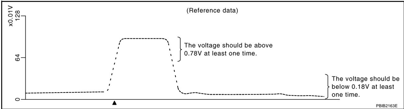
"HO2S2 (B1)/(B2)" should be above 0.78V at least once when the "FUEL INJECTION" is +25%.
