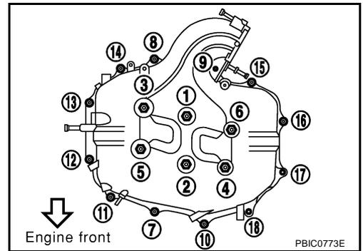
9. Remove PCV hose [between intake manifold collector (lower) and rocker cover (right bank)].
