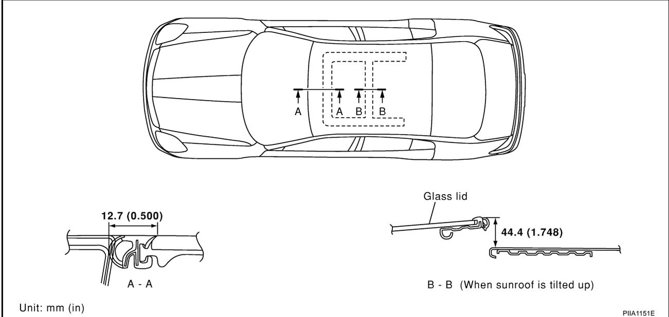
3. If necessary, adjust height difference by using the following procedure.
