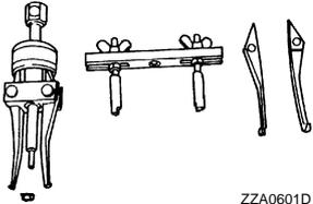
ZZA0601D<br><ul style="list-style-type: none"> <li>● Removing rear oil seal</li> </ul>                                             |
