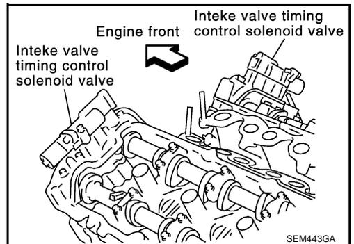
4. Remove intake and exhaust camshaft brackets.
