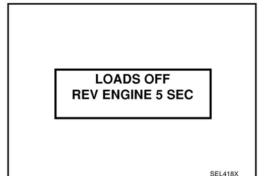
7. The tester now checks the engine at idle and performs the DIODE/RIPPLE check.
