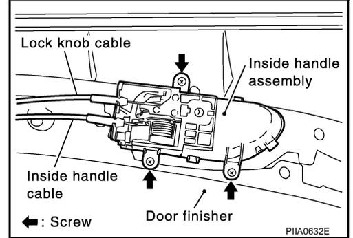
3. Remove the mounting bolts (TORX T30), remove the door lock assembly.
