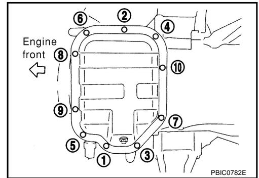
4. Install oil pan drain plug.
