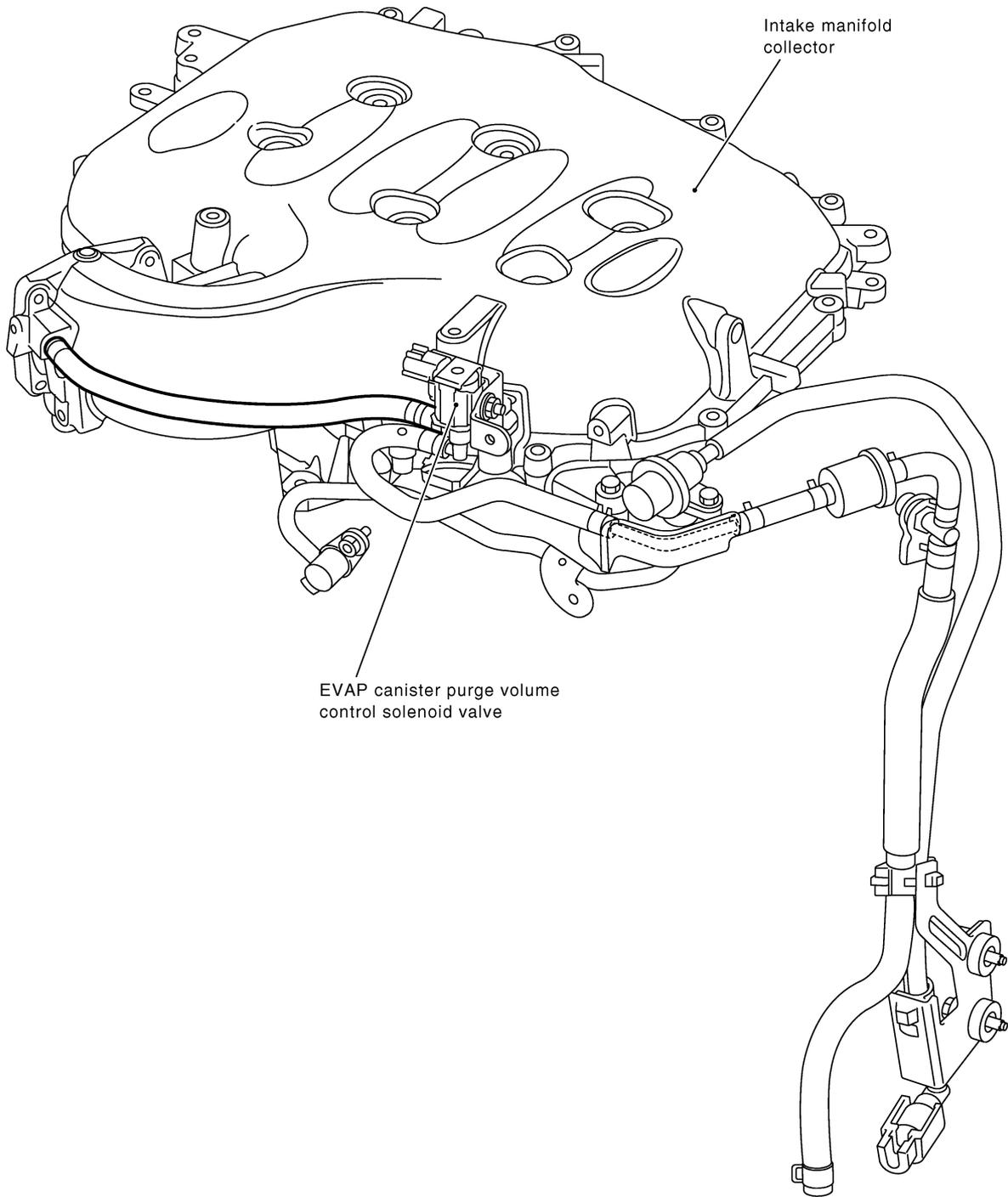
**NOTE:** Do not use soapy water or any type of solvent while installing vacuum hose or purge hoses.
