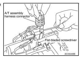
42. Disconnect TCM connector and park/neutral position switch connector.
