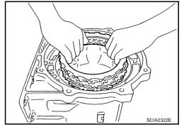
52. Remove snap ring (fixing spring retainer) using a flat-bladed screwdriver.
