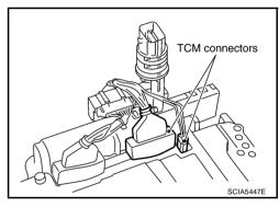
d. Install O-ring to A/T assembly harness connector.
