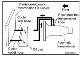
5. Insert the extension adapter hose of a can of Transmission Cooler Cleaner (Nissan P/N 999MP-AM006) into the cooler outlet hose.
