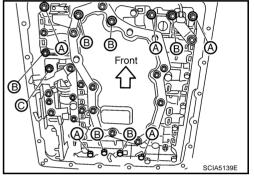
7. Tighten bolt 1, 2 and 3 temporarily to prevent dislocation. After that tighten them in order  $(1 \rightarrow 2 \rightarrow 3)$ , and then tighten other bolts.
