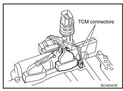
20. Remove A/T assembly harness connector from control valve with TCM using a flat-bladed screwdriver.
