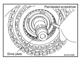
35. Install high and low reverse clutch hub, mid sun gear assembly and rear sun gear assembly as a unit.
