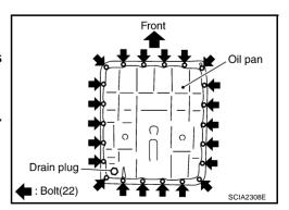
Tighten oil pan mounting bolts to the specified torque in numerical order shown in the figure after temporarily tightening them.
