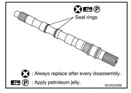
27. Install parking gear to output shaft.
