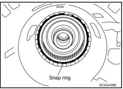
18. Measure clearance between retaining plate and snap ring. If not within specified clearance, select proper retaining plate.
