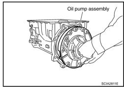
4. Apply recommended sealant (Genuine RTV Silicone Sealant or equivalent. Refer to <u>GI-46</u>, "<u>Recommended Chemical Products and Sealants</u>" .) to oil pump assembly as shown in illustration.
