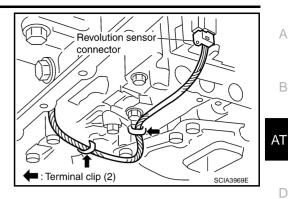
14. Remove revolution sensor from transmission case.
