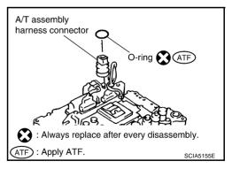
Install A/T fluid temperature sensor 2 to bracket.
