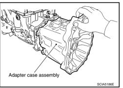
Tighten adapter case assembly mounting bolts to specified torque. (With bracket.)
