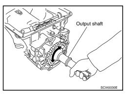
29. Install bearing race to output shaft.
