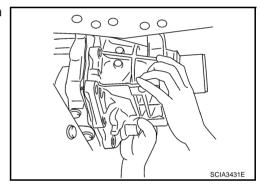
9. Remove bearing race from output shaft.
