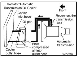
Radiator/Automatic Transmission Oil Cooler Front Cooler Reconnect the inlet hose transmission Oil pan lines Automatic transmission Transmisson Coólei Cooler outlet hose Cleaner SCIA3831F
