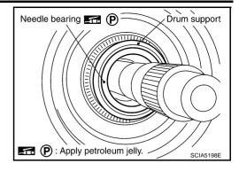
33. Install high and low reverse clutch assembly in direct clutch.
