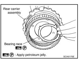
38. Install rear carrier assembly in direct clutch drum.
