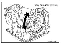
47. Install needle bearing to front sun gear.
