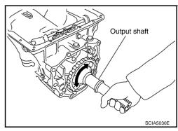
46. Remove parking gear from output shaft.
