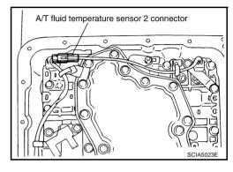
7. Straighten terminal clip to free A/T fluid temperature sensor 2 harness.
