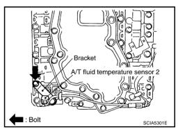
38. Remove bracket from A/T fluid temperature sensor 2.
