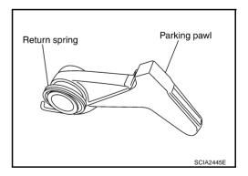
23. Install parking pawl (with return spring) and pawl shaft to rear extension (2WD models) or adapter case (AWD models).
