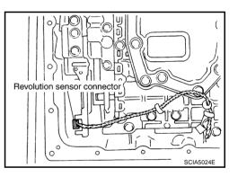
13. Straighten terminal clips to free revolution sensor harness.
