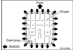
Tighten oil pan mounting bolts to the specified torque in numerical order shown in the figure after temporarily tightening them.
