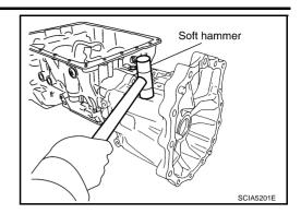
iii. Remove adapter case assembly from transmission case. (With needle bearing)
