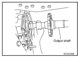
11. Remove parking gear from output shaft.
