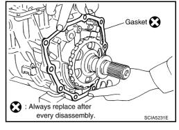
Install adapter case assembly to transmission case.
