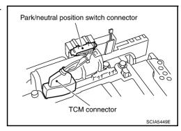
b. Install A/T assembly harness connector from control valve with TCM.
