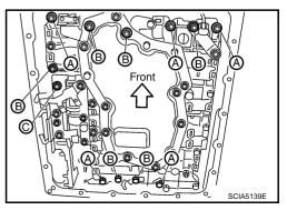
15. Remove control valve with TCM from transmission case.
