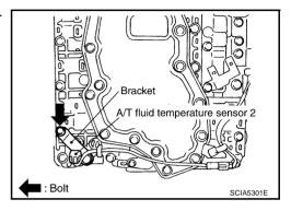
17. Remove bracket from A/T fluid temperature sensor 2.
