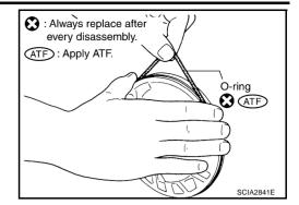
4. Remove O-ring from oil pump cover.
