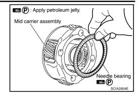
40. Install needle bearing (front side) to mid carrier assembly. **CAUTION:**
