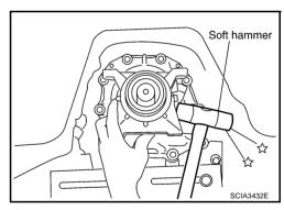
11. Remove rear extension assembly from transmission case. (With needle bearing.)
