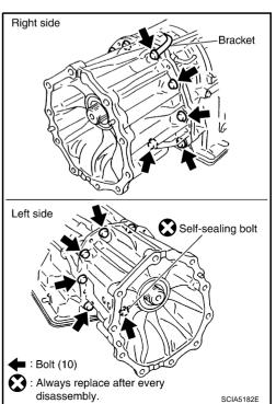
ii. Tap adapter case assembly with soft hammer.
