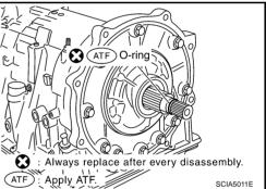
7. Install converter housing to transmission case.
