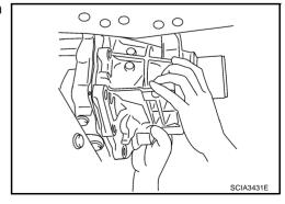
12. Disconnect revolution sensor connector.
