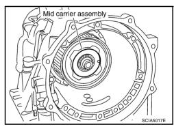
42. Install front carrier assembly, input clutch assembly and rear internal gear as a unit.
