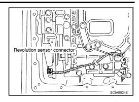
13. Securely fasten revolution sensor harness with terminal clips.
