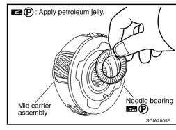
41. Install mid carrier assembly in rear carrier assembly.
