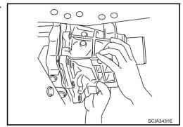
6. Tighten rear extension assembly mounting bolts to specified torque.
