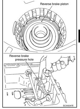
57. Remove lip seal and D-ring from reverse brake piston.
