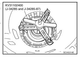
15. Install reverse brake retaining plate, drive plates, driven plates and dish plate in transmission case.
