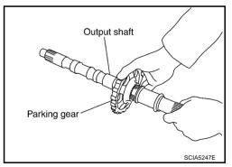
28. Install output shaft in transmission case.
