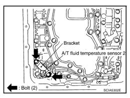
9. Remove bracket from A/T fluid temperature sensor 2.
