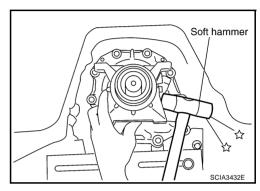
8. Remove rear extension assembly from transmission case. (With needle bearing.)
