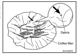
b. If one or more pieces of debris are found that are over 1mm (0.040 in) size and/or peeled clutch facing material is found in the coffee filter, the fluid cooler is not serviceable. The A/T fluid cooler/radiator must be replaced and the inspection procedure is ended.Refer to CO-13, "RADIATOR", CO-16, "RADIATOR (ALUMINUM TYPE)".
