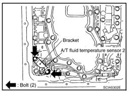
Connect A/T fluid temperature sensor 2 connector.
