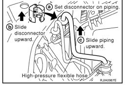
Remove mounting nut for high-pressure flexible hose, and then remove high-pressure flexible hose.
