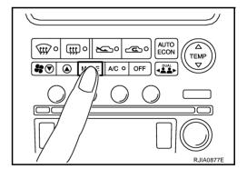
3. Confirm that discharge air comes out according to the air distribution table. Refer to <a href="ATC-36">ATC-36</a>, "Discharge Air Flow"</a>.
