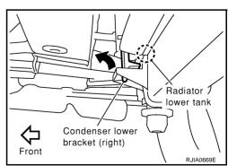
Pull condenser forward at an angle. Remove condenser from radiator.
