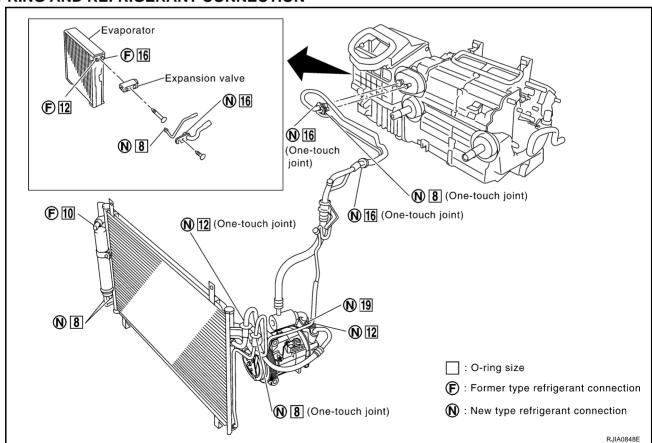
The new and former refrigerant connections use different O-ring configurations. Do not confuse Orings since they are not interchangeable. If a wrong O-ring is installed, refrigerant will leak at, or around, the connection.
