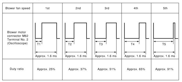
NOTE: Duty ratio =  $\frac{1 \text{ x}}{\text{Approx. 1.6 ms}} \times 100 \text{ (%)}$
