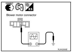
3. Vary the fan speed between Lo and Hi and confirm the duty ratios between blower motor harness connector M62 terminal 2 (G) and ground using an oscilloscope. Usual terminal 2 (G) drive signal duty ratios are shown in the table below.
