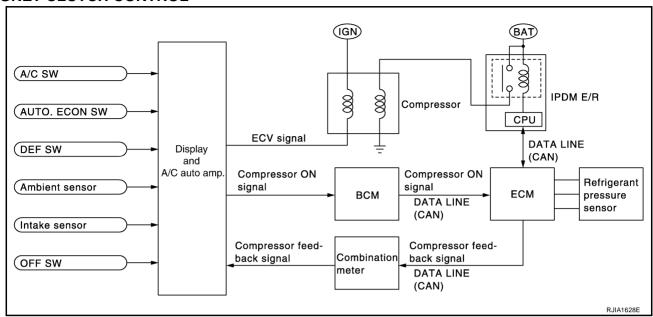
When A/C switch, AUTO.ECON switch or DEF switch is pressed, display and A/C auto amp. inputs compressor ON signal to BCM.
