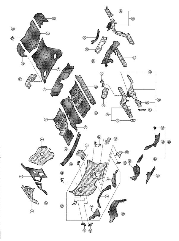
\* Indicates both sided anti-corrosive precoated steel portions \* Indicates aluminum portion
