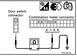
4. Check continuity between door switch connector B17, B23, B20, B32 terminals 1 and ground.
