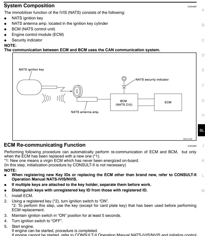
If engine cannot be started, refer to CONSULT-II Operation Manual NATS-IVIS/NVIS and initialize control unit.
