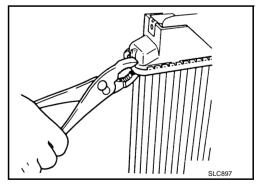
4. Make sure that the rim is completely crimped down.
