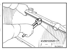
• Grip the crimped edge and bend it upwards so that radiator plate pliers B slips off.
