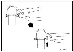
• In areas where radiator plate pliers B cannot be used, use flat-bladed screwdriver to bend the edge up.
