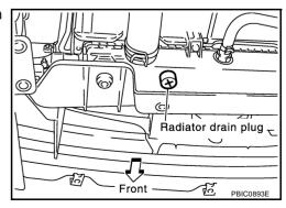
When drain all of engine coolant in the system, open drain plugs on engine cylinder block. Refer to <a href="EM-122">EM-122</a>, "DISASSEMBLY"</a>.
