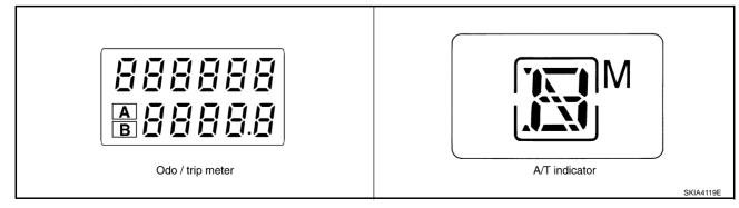
7. Push the odo/trip meter switch. Each meter/gauge should indicate as shown in the figure while pushing odo/trip meter switch. (At this time, the low-fuel warning lamp goes off).
