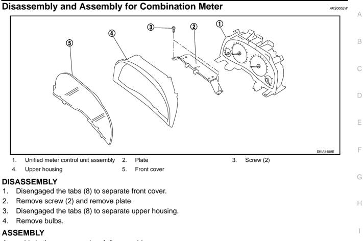
Assembly in the reverse order of disassembly.
