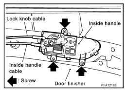
8. Disconnect metal clips and pawls from door finisher back side, and remove power window switch finisher.
