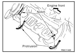
b. Apply liquid gasket to oil pan gaskets as shown in the figure. Use Genuine RTV Silicone Sealant or equivalent. Refer to GI-46, "RECOMMENDED CHEMICAL PRODUCTS AND SEALANTS".
