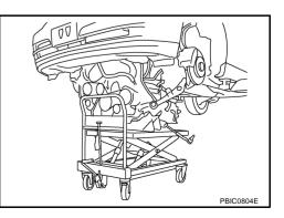
2. Remove rear engine mounting member bolts.
