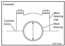
Remove main bearing caps and bearings, and using scale on Plastigage bag, measure the Plastigage width. NOTE:
