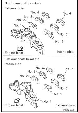
• Install camshaft brackets (No. 2 to No. 4) aligning the stamp marks as shown in the figure.
