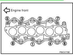
5. Remove intake manifold gaskets.
