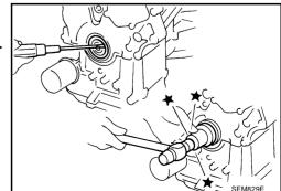
3. Remove front oil seal using suitable tool.
