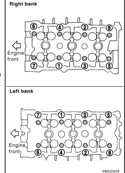
d. Turn all bolts 90 to 95 degrees clockwise [target: 90 degrees (angle tightening)].
