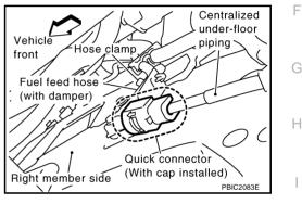
c. Disconnect quick connector from centralized under-floor piping as follows: CAUTION:
