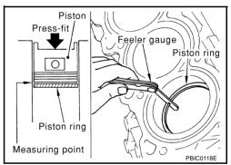
• If the measured value exceeds the limit, replace piston ring, and measure again. If it still exceeds the limit, re-bore cylinder and use oversize piston and piston rings.
