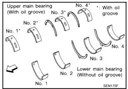
• Main bearing caps are identified by identification mark cast on them. For installation, face front mark to front side.
