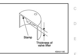
Available thickness of valve lifter: 27 sizes with range 7.88 to 8.40 mm (0.3102 to 0.3307 in) in steps of 0.02 mm (0.0008 in) (when manufactured at factory). Refer to <u>EM-153</u>, "Available Valve Lifter".
