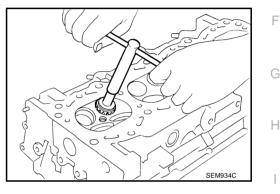
Grind to obtain the dimensions indicated in the figure. Exhaust side Ē. mm 0.051 - 0.059 60 - 1.51 -89 89.5 45 D2 dia. : 36.6 - 36.8 mm (1.441 - 1.449 in)<sup>\*2</sup> 53 12Ò
