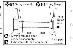
• Install axle pipe to oil pan from axle pipe flange side (LH side) using a suitable drift [43 - 57 mm (1.69 - 2.24 in)]. **CAUTION:**
