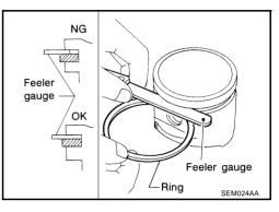
• If the measured value exceeds the limit, replace piston ring, and measure again. If it still exceeds the limit, replace piston also.
