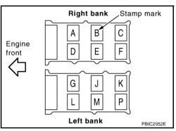
Apply sealant to mating surface of camshaft brackets (No. 1) as shown on right and left banks.
