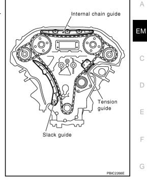
27. Remove timing chain (primary) and crankshaft sprocket.
