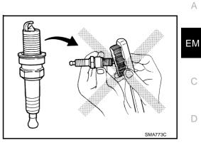
• Checking and adjusting plug gap is not required between change intervals.
