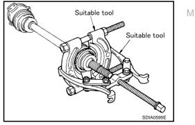
4 Screw a drive shaft puller (suitable tool) 30 mm (1.18 in) or more into threaded part of joint sub-assembly. Pull joint sub-assembly out of shaft.
