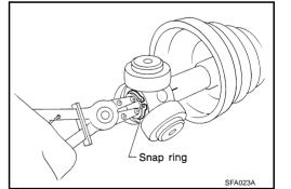
Serration chamfer facing shaft 7. Install housing to spider assembly. Apply Nissan genuine grease or equivalent to housing.
