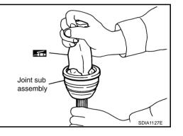
3. Wind serrated part of shaft with tape. Install boot band and boot to shaft. Be careful not to damage boot.
