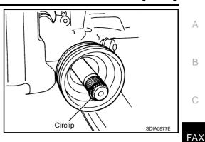
18. Insert the amount grease (Nissan genuine grease or equivalent) into joint sub-assembly serration hole until grease begins to ooze from ball groove and serration hole. After inserting grease, use a shop cloth to wipe off old grease that has oozed out.
