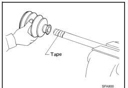
5. Attach circular clip to shaft. At this time, circular clip must fit securely into shaft groove. Attach nut to joint sub-assembly. Use a wooden hammer to press-fit.
