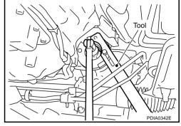
Put a matchmark on the end of the drive pinion corresponding to the B position matchmark on the final drive companion flange.
