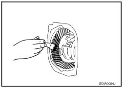
4. Check the tooth contact on both sides (drive side and coast side).
