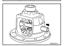
Turn the pinion mate gear, then remove the pinion mate gear, pinion mate thrust washer, side gear and side gear thrust washer from the differential case.
