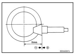
2. If there is heel contact or face contact, increase point height adjusting washer in order to bring drive pinion close to drive gear.
