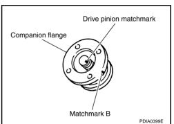
4. Remove the companion flange using puller (commercial service tool).
