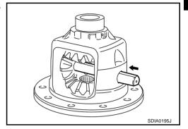
6. Place the differential gear case so that measurement point facing up as shown.
