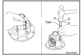
13. Apply genuine medium strength locking sealant or equivalent to the drive gear bolt hole thread. Refer to GI-46, "Recommended Chemical Products and Sealants".
