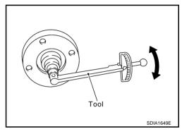
If the preload value is out of standard, adjust pinion bearing preload and side bearing preload. Refer to
