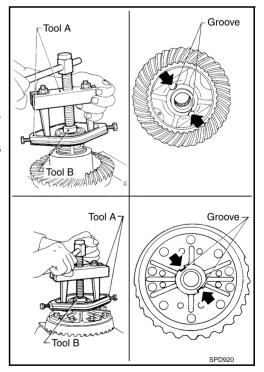
• Be careful not to confuse left-hand and right-hand parts. Keep bearing and bearing race for each side together.
