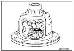
d. Check mating surfaces of differential case, side gears, pinion mate gears, pinion mate shaft and thrust washers.
