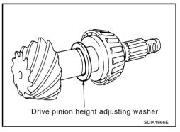
3. If the hypoid gear set has been replaced, select the adjusting washer.
