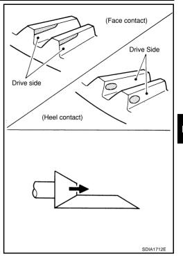
3. If there is toe contact or flank contact, decrease pinion adjusting washer in order to make drive pinion go away from drive gear.
