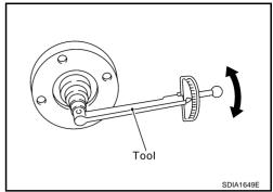
• If the preload value is out of standard, adjust preload by changing adjusting shim thickness (side retainer side). Refer to FFD-33, "Side Bearing Adjusting Shims".
