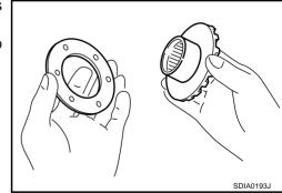
Install the side gear, thrust washers, pinion mate gears and thrust washers to differential case.
