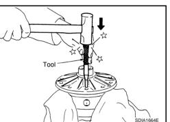
b. Remove the pinion mate shaft.
