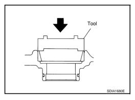
2. Install side bearing outer race into the side retainer with tool.
