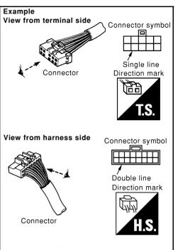
Male and female terminals Connector guides for male terminals are shown in black and female terminals in white in wiring diagrams.
