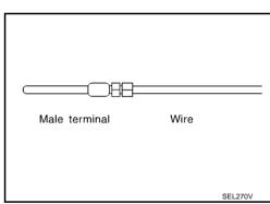
While holding the wire of the male terminal, try to insert the male terminal into the female terminal.
