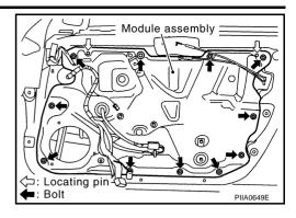
7. Draw out the locating pins on the upper of the module assembly from the door panel, and then remove the module assembly by drawing forward and moving upward.
