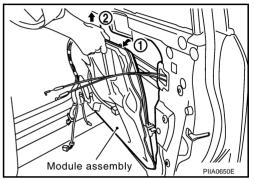
8. Disconnect the harness connector for the module assembly, and unclip the harness from the back.
