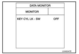
Check door key cylinder switch ("KEY CYL UN-SW") in "DATA MONITOR" mode for "POWER DOOR LOCK SYSTEM" with CONSULT-II. Refer to <u>BL-31</u>, "<u>Data Monitor</u>"
