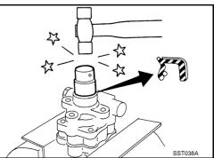
4. Set dowel pin at the illustration position (The position is the same regardless of right or left direction), and install side plate to body assembly.
