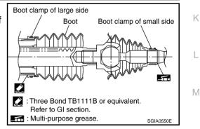
Tighten large-diameter side of RH/LH boot with boot clamp a. (stainless wire).
