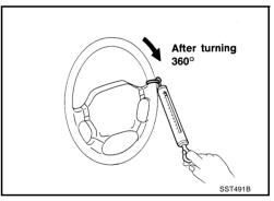
5. If steering wheel turning force is out of specification, check relief oil pressure of oil pump. Refer to <u>PS-25</u>, <u>"POWER STEERING OIL PUMP"</u>.
