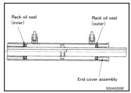
a. To avoid damaging inner rack oil seal, wrap an OHP sheet [approximately. 70 mm (2.76 in)  $\times$  100 mm (3.94 in] around rack tooth. Place oil seal on sheet. Then, pull oil seal along with OHP sheet until they pass the toothed section of rack, then remove it.
