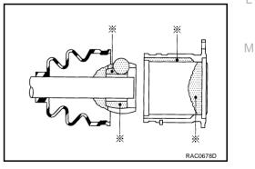
8. Install boot securely into grooves (indicated by \* marks) shown in the figure.
