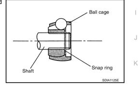
5. Insert the amount grease (NISSAN genuine grease or equivalent) onto housing (\* point) to the quantity mentioned below, and install it to shaft.
