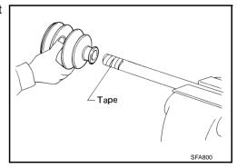
Wind serrated part of shaft with tape. Install boot band and boot to shaft. Be careful not to damage boot.
