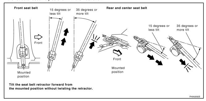
15 degrees or less tilt : Belt can be pulled out.
