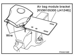
4. Connect deployment tool adapter (SST: J38381-80) to air bag module connector and deployment tool connector [SST: KV99106400 (J38381)].
