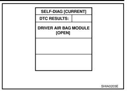
If no malfunction is detected on "SELF-DIAG [CURRENT]" even though malfunction is detected in "SRS Operation Check", check the battery voltage. If the battery voltage is less than 9 V, charge or replace the battery. Then go to SRS-24, "DIAGNOSTIC PROCE-DURE 3" . If the battery voltage is OK, go to SRS-26, "DIAGNOSTIC PROCEDURE 4 (CONTINUED FROM DIAGNOSTIC PROCEDURE 2)" to diagnose the following cases:
