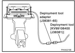
7. Press the button on the deployment tool. The left side lamp on the tool, marked "air bag connector voltage", will illuminate and the air bag module will deploy.
