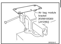
3. Match the hole in air bag module bracket (held in vise) and front passenger air bag module and fix them with one bolt  $[M8 \times 25 - 30 \text{ mm } (0.98 - 1.18 \text{ in})]$ .
