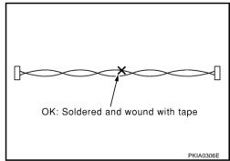
Do not perform bypass wire connections for the repair parts. (The spliced wire will become separated and the characteristics of twisted line will be lost.)
