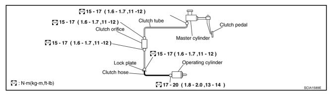
Carefully observe the following steps during clutch tube removal and installation.
