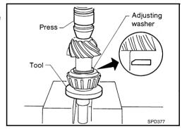
4. Set drive pinion assembly (as shown in figure) in differential carrier and install drive pinion, with press and suitable tool.
