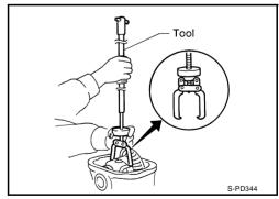
Keep the side bearing outer races together with inner races.
