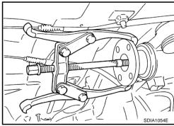
5. Using the side bearing outer race puller, remove oil seal.
