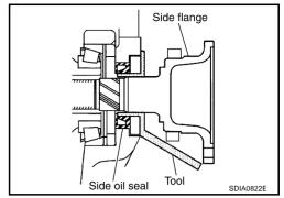
c. Put suitable drift on the center of side flange, then drive it until sound changes.
