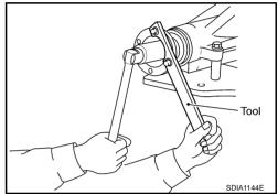
3. Using the puller remove companion flange.
