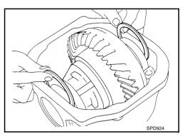
4. Install the side bearing caps in their correct locations and torque the bearing cap retaining bolts.
