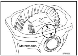
6. Measure the turning torque of the carrier at the ring gear retaining bolts with a spring gauge, J-8129.
