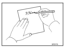
4. Correct the pinion height washer size by referring to the "pinion head number".
