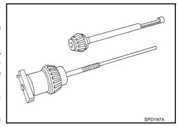
Install the pinion rear bearing inner race into the final drive housing. Then place the pinion preload shim selector Tool, J34309-1, gauge screw assembly.
