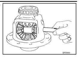
3. Adjust clearance between rear face of side gear and thrust washer by selecting side gear thrust washer. Refer to RFD-34. "AVAILABLE SIDE GEAR THRUST WASHERS".
