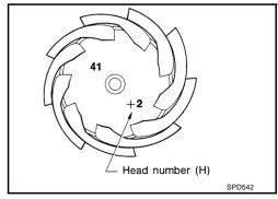
There are two numbers painted on the drive pinion gear. The first one refers to the drive pinion and ring gear as a matched set. This number should be the same as the number on the ring gear. The second number is the "pinion head height number". It refers to the ideal pinion height from standard for quietest operation. Use the following chart to determine the correct pinion height washer.
