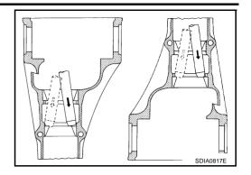
9. Remove pinion rear bearing inner race and drive pinion height adjusting washer with Tool.
