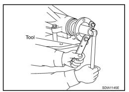
Tighten the drive pinion nut by very small degrees until the specified preload in achieved, when checking the preload, turn drive pinion in both directions several times.
