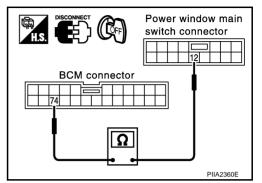
3. Check continuity between BCM connector M3 terminal 74 and power window sub-switch (door lock and unlock switch) connector D37 terminal 16.
