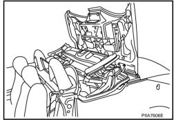
6. Remove the dove tail female mounting nuts. Remove the dove tail female.
