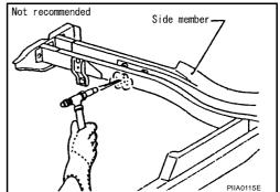
When straightening body panels, use caution in pulling any HSS panel. Because HSS is very strong, pulling may cause deformation in adjacent portions of the body. In this case, increase the number of measuring points, and carefully pull the HSS panel.
