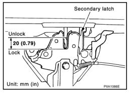
Check the hood lock lubrication condition. If necessary, apply "body grease" to the points shown in the figure.
