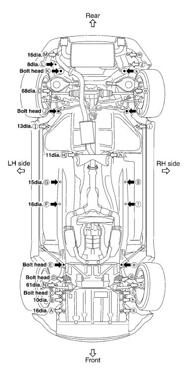
(A),(a) ①,① X:413 X:605 Y:-368 Y:2191 Z:305 Z:128 **B**,**b**  $\bigcirc$ , $\bigcirc$ X:415 X:473 Y:-238 Y:2404 Z:274 Z:114 (C),(C) (k),(k)X:405 X:452 Y:-100 Y:2964 Z:225 Z:179 (D),(d) (L) X:405 X:550 Y:39 Y:3065 Z:224 Z:316 E,e Ø X:-500 X:388 Y:279 Y:3073 Z:82 Z:316 (F),(f) (M), (m)X:438 X:533 Y:3275 Y:1100 Z:79 Z:316 (G),(9) X:440 Y:1400 Z:79  $\mathbb{H}$ , $\mathbb{h}$ X:205 Y:1777 Z:69
