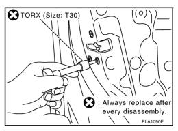
Remove the outside handle mounting bolts, remove the outside handle.
