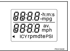
5. Push the odo/trip meter switch. Each meter/gauge should indicate as shown in the figure while pushing odo/trip meter switch.
