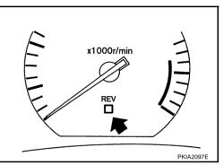
reaches the set figure. The figure of engine speed can changed between 2,000 and 8,000 rpm by pressing trip computer setting switch. Pressing the trip computer setting switch for less than approximately 1 second will add the figure by 100 rpm. If pressing for more than approximately 1 second, the figure will increase by 500 rpm.
