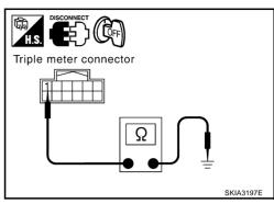
3. Check continuity between unified meter and A/C amp. harness connector M49 terminals 29 (B), 30 (B) and ground.
