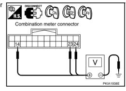
3. Check voltage between unified meter and A/C amp. harness connector terminals and ground.
