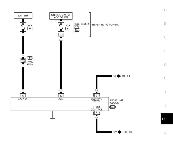
REFER TO THE FOLLOWING. (E108) -SUPER MULTIPLE JUNCTION (SMJ) (M4) -FUSE BLOCK-JUNCTION BOX (J/B)
