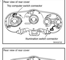
5. Remove screws (2) and remove rear cover.
