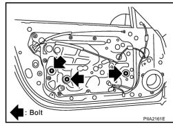
4. While holding door window, raise it at rear end to pull the glass out of sash toward outside of door.
