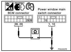
4. Check continuity between BCM connector M1 terminal 28, power window sub-switch connector D37 terminal 10, and between BCM connector M1 terminal 28 and ground.
