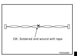
Do not perform bypass wire connections for the repair parts. (The spliced wire will become separated and the characteristics of twisted line will be lost.)
