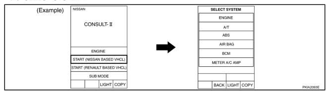
Print all the data of "SELF-DIAG RESULTS" for "ENGINE", "A/T", "METER A/C AMP", "BCM", and "ABS" displayed on CONSULT-II.
