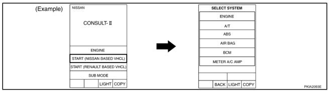
2. Print all the data of "SELF-DIAG RESULTS" for "ENGINE", "METER A/C AMP", "BCM", and "ABS" displayed on CONSULT-II.
