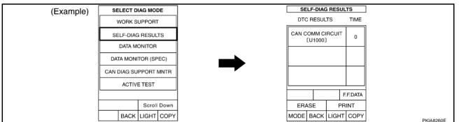
3. Print all the data of "CAN DIAG SUPPORT MNTR" for "ENGINE", "A/T", "METER A/C AMP", "BCM", and "ABS" displayed on CONSULT-II.
