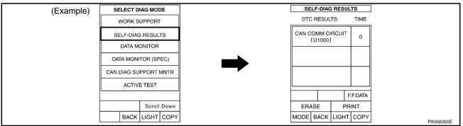
3. Print all the data of "CAN DIAG SUPPORT MNTR" for "ENGINE", "METER A/C AMP", "BCM", and "ABS" displayed on CONSULT-II.
