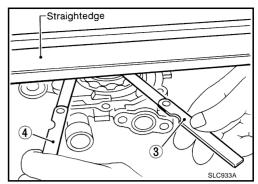
Calculate the clearance between inner rotor and oil pump body as follows.
