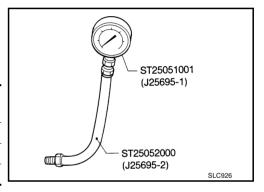
If difference is extreme, check oil passage and oil pump for oil leaks.
