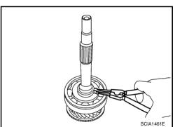
Set the suitable puller on the main drive gear and then using a press to remove main drive gear bearing from the main drive gear.
