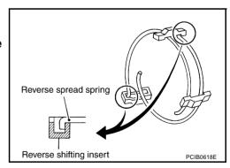
26. After installing reverse main gear bushing, reverse main needle bearing, reverse main gear, and reverse baulk ring onto the main shaft, using the drift and press plate and a press to press fit the reverse synchronizer assembly.
