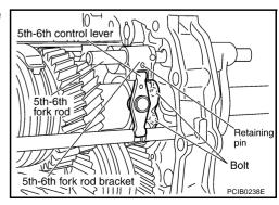
16. Using a pin punch [6 mm (0.24 in) dia.] to knock out retaining pin, and then remove 5th - 6th fork rod bracket and 5th - 6th fork rod.
