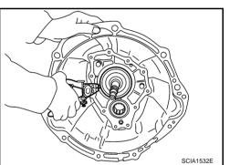
20. Using a soft hammer to carefully tap main shaft and counter shaft from the transmission case side, and then separate adapter plate and transmission case.
