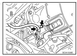
13. Remove crankshaft position sensor (POS).
