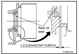
17. Apply Genuine Silicone RTV or equivalent refer to GI section to the adapter plate rear extension mounting surface as shown in the figure.
