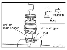
10. Install 3rd - 4th main spacer on the main shaft and then using the inserter and a press to press fit the 4th main gear.
