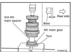
11. Using the inserter and a press to press fit the main shaft bearing onto the main shaft.
