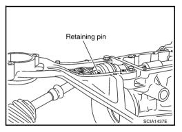
6. Remove control bracket mounting bolts. Then remove check shift pin and control bracket as one unit from the rear extension.
