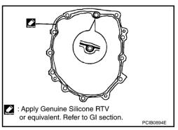
18. Install rear extension to the adapter plate and then tighten mounting bolts to the specified torque in order as shown on the figure.
