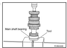
12. Using the inserter and a press to press fit the reverse main gear bushing onto the main shaft.
