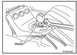
d. Turn monkey wrench with water pump plier and others fixed. Loosen shift knob, and remove shift knob from control lever assembly.
