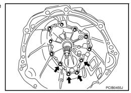
11. Tighten bolts to the specified torque in order as shown on the figure.
