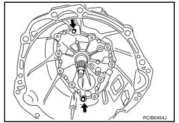
10. Temporary tightening remaining 9 bolts, tighten bolts to the specified torque.
