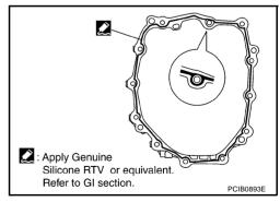
Place the adapter plate in the transmission case, using soft hammer to tap the adapter plate to install it into the transmission case.
