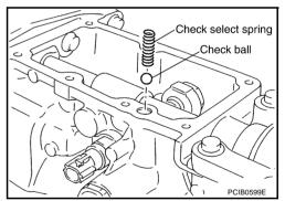
25. Install rear extension upper cover gasket and rear extension upper cover to rear extension.
