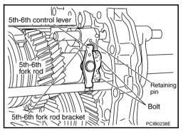
7. Install 5th - 6th control lever to the adapter plate and then tighten mounting bolts to the specified torque.
