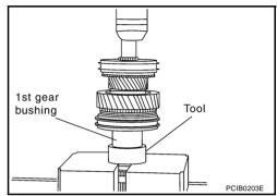
Install 1st outer baulk ring, 1st synchronizer cone, 1st inner baulk ring, 1st needle bearing, and 1st main gear on the main shaft and then using the inserter and a press to press fit the 3rd main gear.
