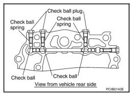
6. Remove 3rd - 4th control lever mounting bolts and then remove 3rd - 4th control lever and shifter cap.
