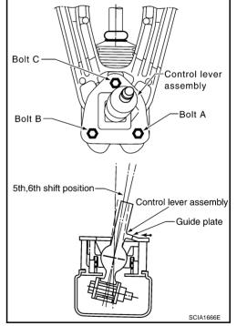
11. As shown in the figure, assemble seat and insulator to control lever assembly.
