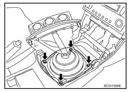
11. Remove guide plate mounting bolts and then separate shift lever assembly from the shift lever housing assembly.
