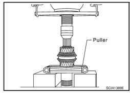
21. Using a press to remove the 3rd gear bushing.
