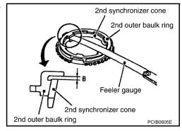
3. Using filler gauge put and press baulk ring on 2nd main gear taper cone, and then measure "clearance C" at more then 2 diagonal points, and calculate the average.
