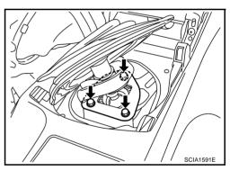
12. Remove clutch operating cylinder mounting bolts and then separate clutch operating cylinder from the transmission case.
