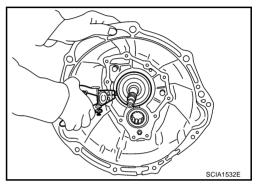
6. Tighten baffle plate mounting nut to the specified torque.
