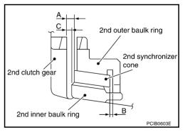
1. Using feeler gauge put and press baulk ring on 2nd main gear taper cone, and then measure "clearance A" at more then 2 diagonal points, and calculate the average.
