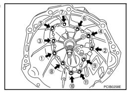
12. Install washer to the withdrawal lever ball pin and then install it to front cover. Tighten withdrawal lever ball pin to the specified torque.
