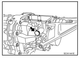
8. Remove rear oil seal from the rear extension using an oil seal puller.
