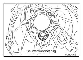
3. Apply Genuine Silicone RTV or equivalent refer to GI section to the transmission case adapter plate mounting surface as shown in the figure.
