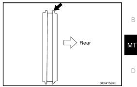
2. Install 5th - 6th spread spring in the 5th - 6th shifting insert.
