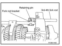
9. Using a pin punch [6 mm (0.24 in) dia.] to knock out retaining pin, and then remove 3rd - 4th shift fork and 3rd - 4th fork rod (reversal side).
