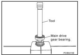
20. Select and install a snap ring to the main drive gear bearing so that the end play comes within the standard value.
