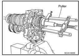
3. Remove main shaft bearing retainer mounting bolts and then remove main shaft bearing retainer.
