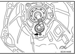
7. Apply multi-purpose grease to the lip of the front cover oil seal. Using a drift, to install oil seal approx. 8.55-9.55 mm (0.336-0.376 in) above from the front cover edge surface.
