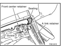
12. Remove screws, and then remove front center retainer.
