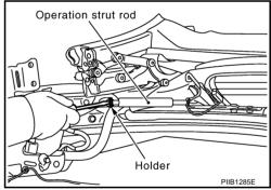
Temporarily fix 5th bow operating strut rods on 5th bow finisher after removal.
