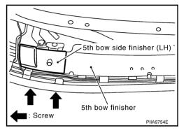
15. Remove 5th bow finisher by pulling the finisher up.
