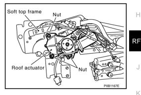
Disconnect 5th bow operating rod (RH/LH) at the frame side by pulling out the holder.
