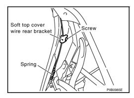
9. Hook soft top cover wire spring on C link and bend the hook of wire spring to prevent unhooking the hook.
