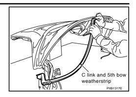
22. Remove screws, and then remove 5th bow retainer.
