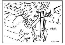
25. Cut EPT seal and remove screws on the bottom of C link. **NOTE:**
