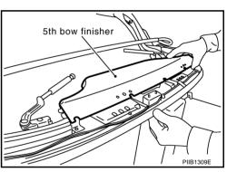
4. Remove rivets head of 5th bow finisher retainer.
