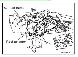
3. Disconnect soft top actuator harness connector.
