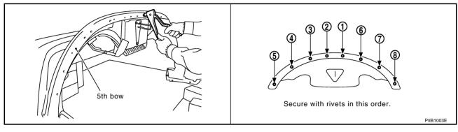
18. Secure soft top cover to C link with rivet.
