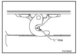
Adjust hook contact length by adjusting front lock rod length using front lock rod adjust bolt if "L" line is not exceeded in front lock hook, RH and LH.
