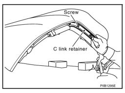
20. Remove clips on the bottom edge of C link and 5th bow weatherstrip.
