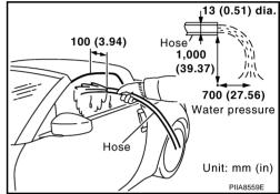
4. Visually check for water leakage.
