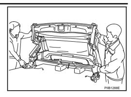
16. Remove clips on the top of C link and 5th bow weatherstrip.
