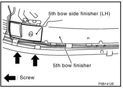
3. Remove clips, and then remove 5th bow finisher.
