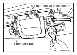
3. Remove bolts, and then remove front lock striker, LH, center, and RH.
