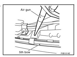
Remove the remains drawn to both ends by the air blow from the gap.
