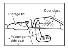
Passenger seatback tilts forward by approximately 6° as soon as windows go down, when soft top switch has been pushed on CLOSE.
