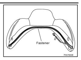
7. Remove the stay fixing the inner cloth.
