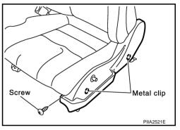
3. Remove screws and remove the power seat switch.
