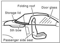
Passenger seatback tilts forward by approximately 6° as soon as windows go down, when soft top switch has been pushed on OPEN.
