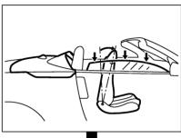
2. Soft top CLOSE operation starts as soon as the passenger seatback tilt forward operation completes.
