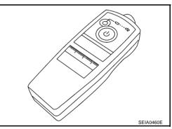
5. Register the IDs in order from FR LH, FR RH, RR RH or RR LH. When ID registration of each wheel has been completed, a buzzer sounds and hazard warning lamp blinks.
