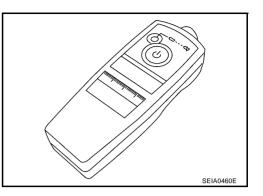
2. Register the IDs in order from FR LH, FR RH, RR RH or RR LH. When ID registration of each wheel has been completed, a hazard warning lamp blinks.
