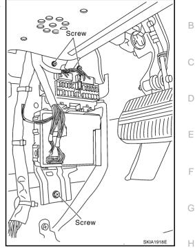
Raise the pawl of fuse block and remove bracket from fuse block to remove BCM.
