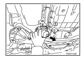
INSTALLATION Installation is the reverse order of removal. CAUTION: Be sure to tighten "B" terminal nut carefully.
