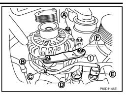
13. Remove alternator assembly downward from the vehicle.
