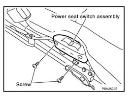
Insert a screwdriver in lower side of power seat switch and remove it (passenger seat for coupe).
