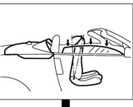
2. Soft top CLOSE operation starts as soon as the passenger seatback tilt forward operation completes.
