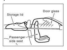
Passenger seatback tilts forward by approximately 6° as soon as windows go down, when soft top switch has been pushed on CLOSE.
