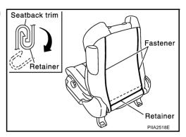
2. Remove the stay securing the inner cloth.
