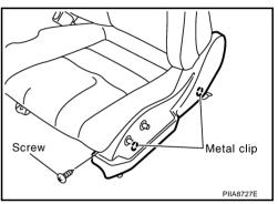
3. Unfasten screws and remove the power seat switch assembly.
