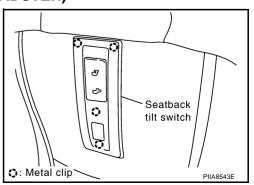
2. Disconnect seatback tilt switch harness connector.
