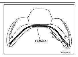
7. Remove the stay securing the inner cloth.
