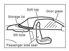
Passenger seatback tilts forward by approximately 6° as soon as windows go down, when soft top switch has been pushed on OPEN.
