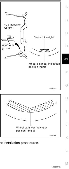
c. If calculated balance weight value exceeds 50 g (1.76 oz), install two balance weight sheets in line with each other as shown.
