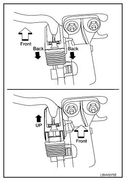
2. Remove the upper and lower accelerator pedal nuts.
