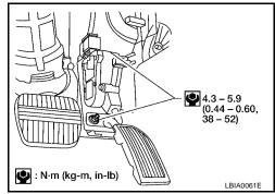
Check that the accelerator pedal moves through the full specified distance of pedal travel.
