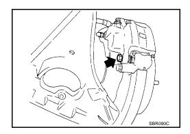
4. Open cylinder body upward and secure with wire. Then remove pad retainers, and inner and outer shims.
