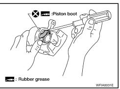
3. Make sure piston boot is properly installed.
