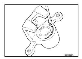
2. Push out piston and piston boot with compressed air.
