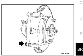
Suspend the cylinder body with wire. Then remove pads with retainers, inner and outer shims and pad return springs.
