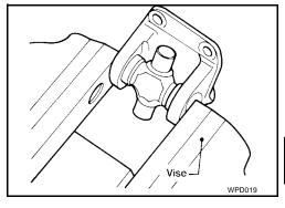
2. Select snap rings that will provide the specified play in an axial direction of the journal, and install them. Refer to <a href="PR-13">PR-13</a>, "Snap Ring".
