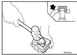
4. Remove the bearing at the opposite side in above operation.
