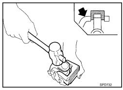
4. Remove the bearing at the opposite side of above operation.
