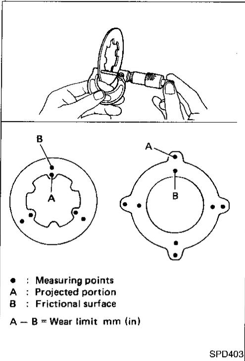
4. Measure frictional surfaces and projected portions of friction discs, plates and spring plate. If any part has worn beyond the wear limit, replace it with a new one that is the same thickness as the projected portion.
