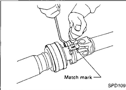
1. Place matching marks on flanges, then separate 2nd tube from 1st tube.
