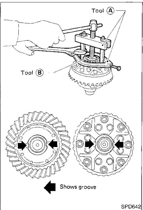
1. Remove side bearing inner cones.
