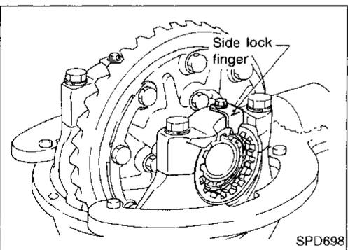
14. Tighten side bearing cap bolts.
