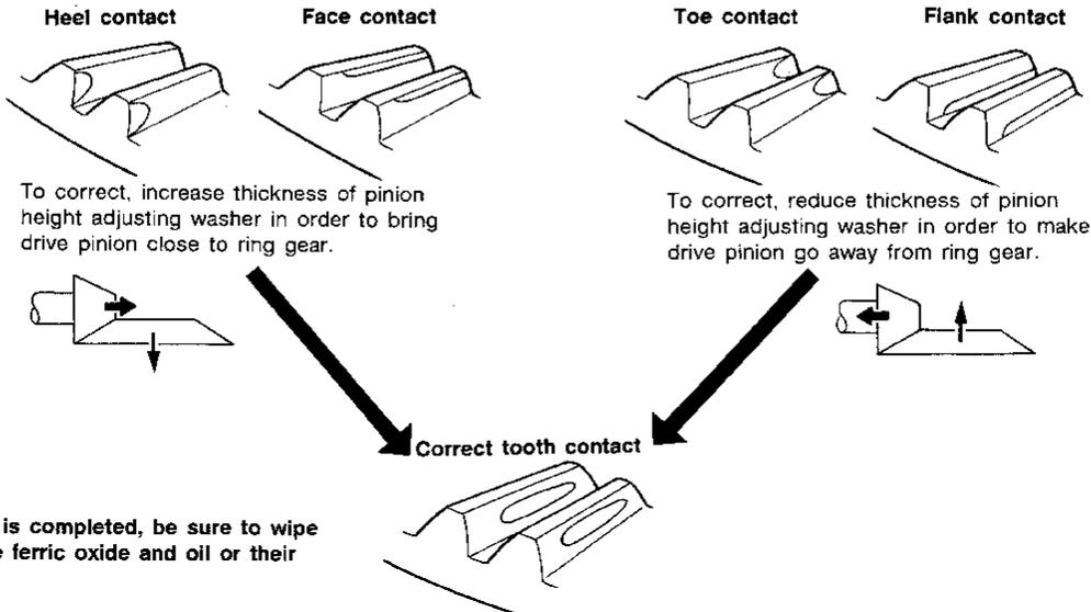
When adjustment is completed, be sure to wipe off completely the ferric oxide and oil or their equivalent.
