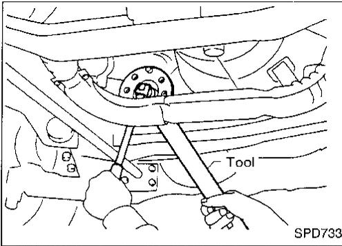
3. Remove companion flange using puller.
