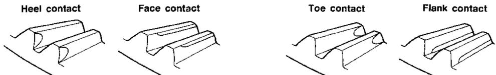
To correct, increase thickness of pinion height adjusting washer in order to bring drive pinion close to ring gear.
