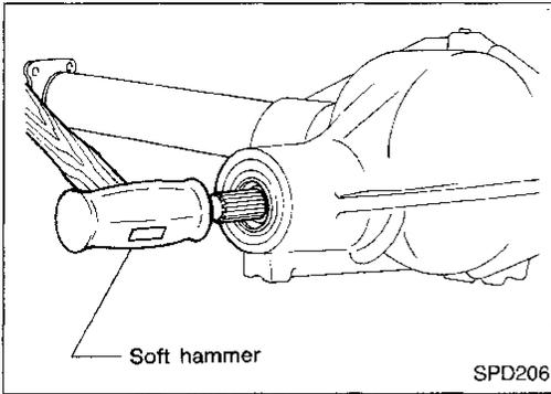
7. Remove drive pinion with soft hammer.
