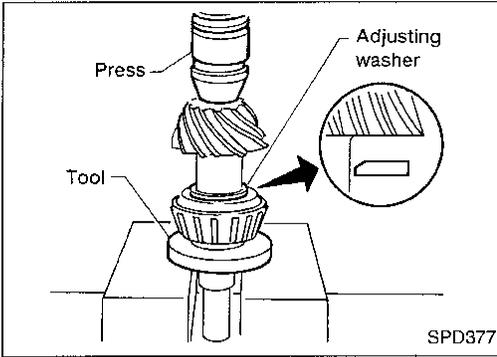
2. Select pinion bearing adjusting washer and drive pinion bearing spacer. Refer to "ADJUSTMENT", PD-25.
