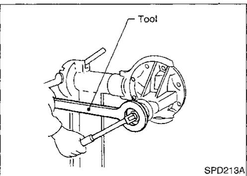
5. Remove drive pinion nut with Tool.
