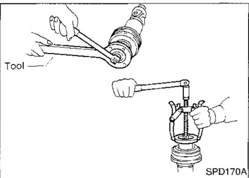
3. Remove locking nut using Tool.
