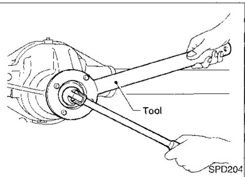
5. Remove pinion nut with Tool.
