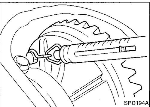
5. Turn the carrier several times to seat the bearings.
