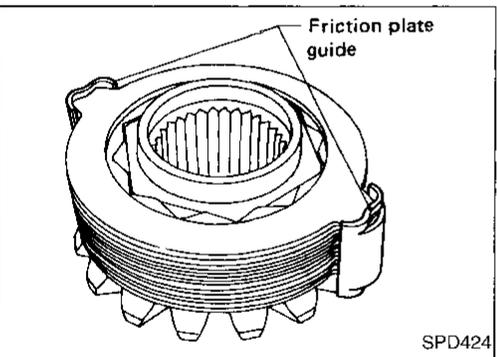
4. Install friction plate guides.
