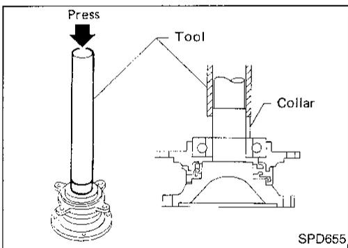
3. Install extension tube retainer, rear axle bearing and rear axle shaft bearing collar on differential side shaft.
