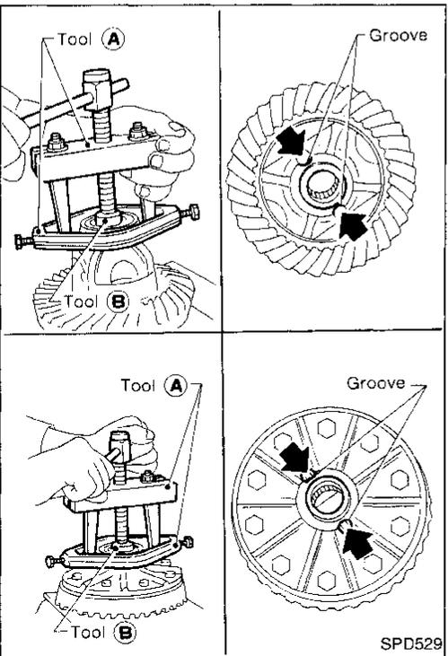
1. Remove side bearing inner cones.
