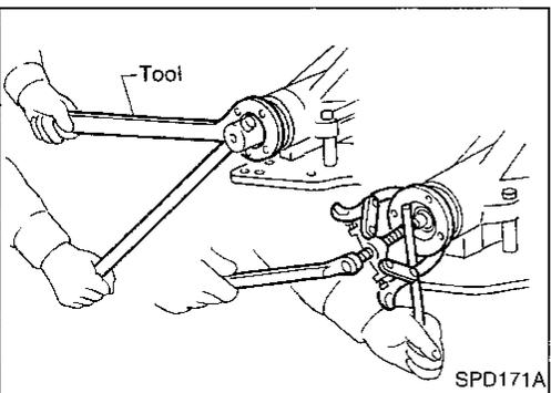
8. Loosen drive pinion nut.
