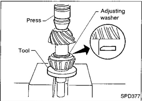
2. Select drive pinion adjusting washer. Refer to "ADJUSTMENT", PD-92.
