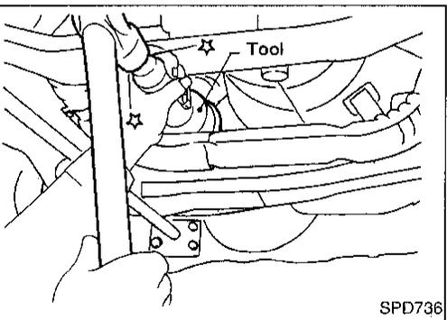
**Front Oil Seal Replacement (Rear final drive: Model H233B)**
