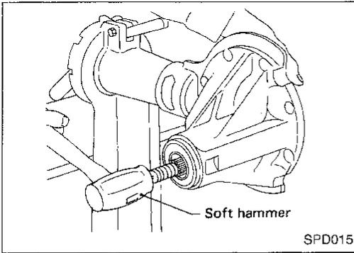
7. Remove drive pinion with soft hammer.
