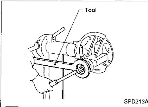
6. Remove drive pinion nut with Tool.
