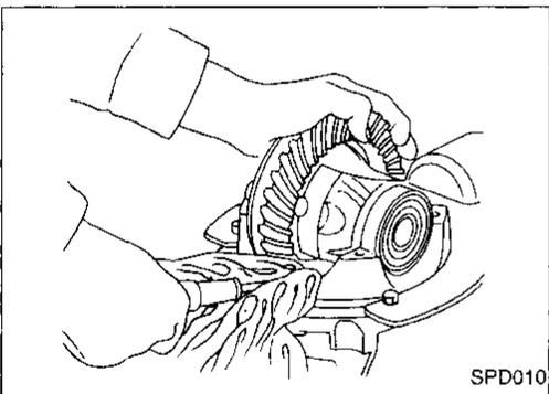
4. Remove differential case assembly with a pry bar.
