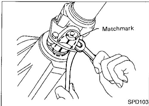
2. Remove propeller shaft.
