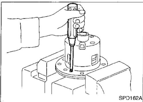
12. Tighten differential case couple screws.
