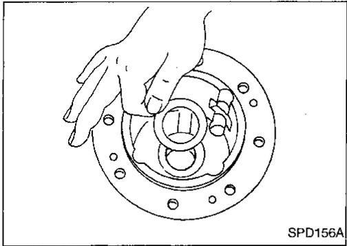
4. Install side gear thrust washer to differential case A.
