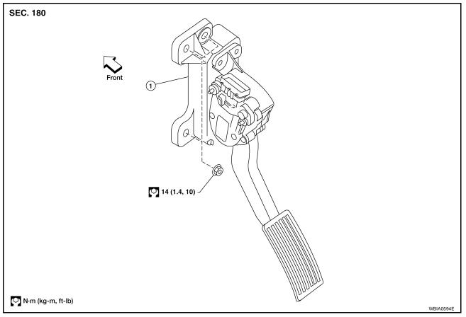
1. Non-adjustable accelerator pedal assembly
