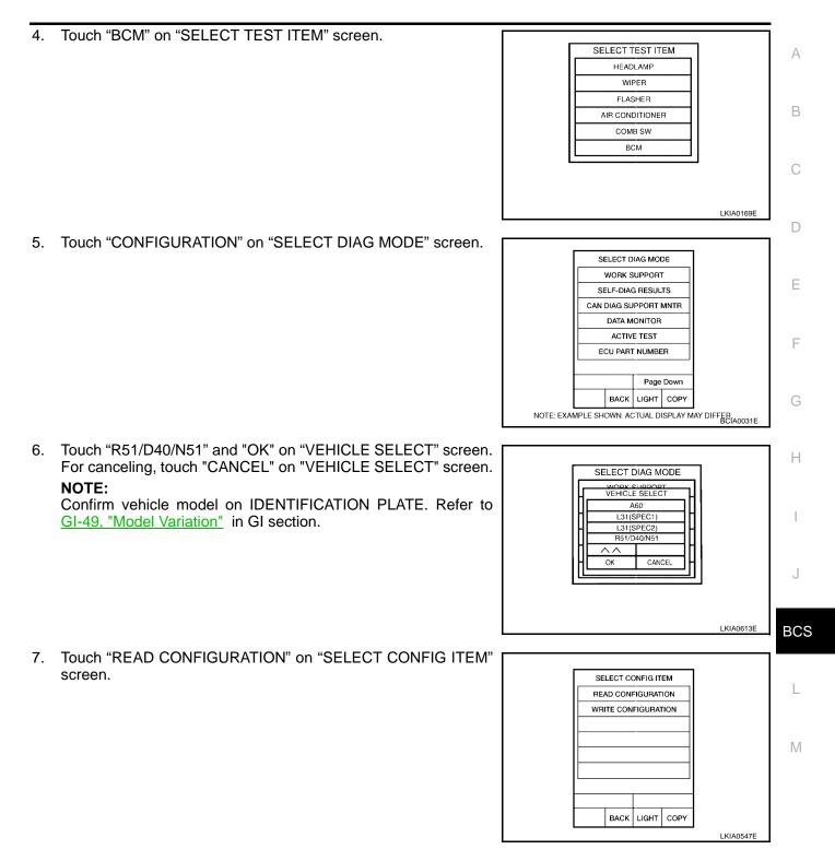
Configuration of current BCM is printed out automatically. A listing of manual setting items and auto setting items will be displayed. Auto setting items are preset and cannot be changed. Manual setting items can be set by using WRITE CONFIGURA-TION PROCEDURE. Refer to <u>BCS-22, "WRITE CONFIGURA-TION PROCEDURE"</u>.
