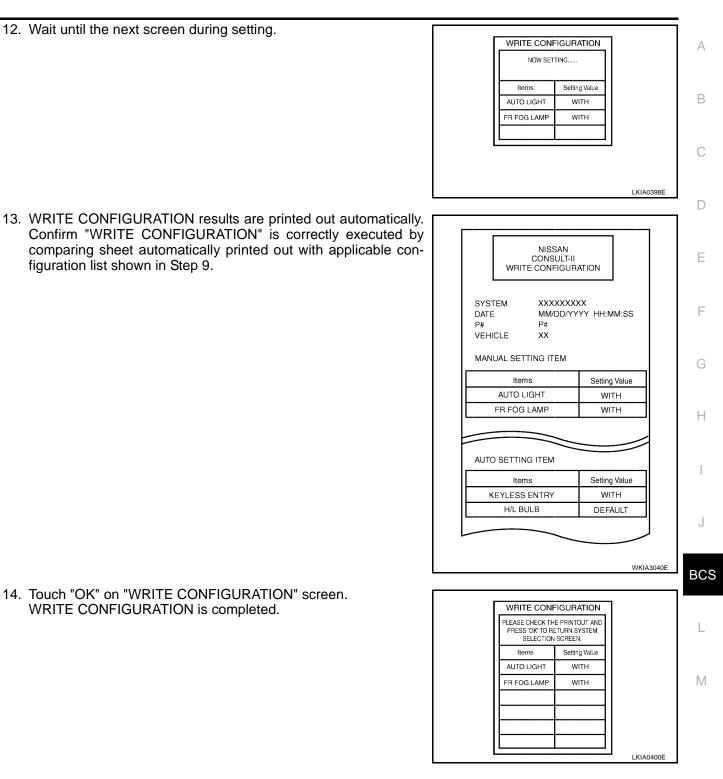
14. Touch "OK" on "WRITE CONFIGURATION" screen. WRITE CONFIGURATION is completed.
