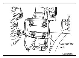
4. Remove the rear spring shackle and bushings using power tool.
