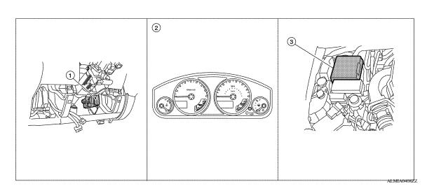
I. BCM M18, M19, M20 (view with low- 2. er instrument panel LH removed)
