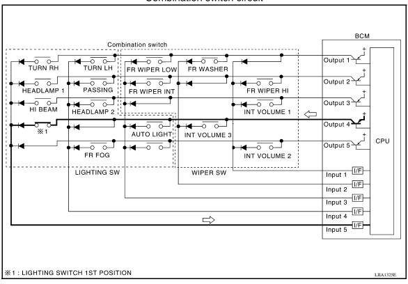
Combination switch INPUT-OUTPUT system list
