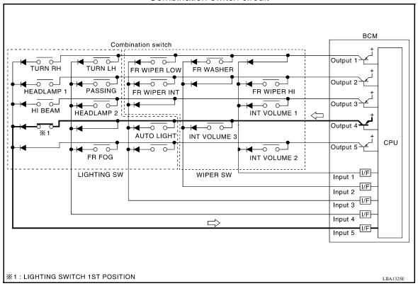
Combination switch INPUT-OUTPUT system list
