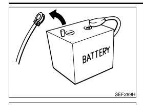
Before starting repairs which do not require battery power: Turn off ignition switch.
