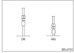
If the male terminal can be easily inserted into the female terminal, replace the female terminal.
