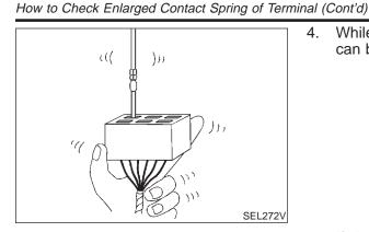
While moving the connector, check whether the male terminal can be easily inserted or not.
