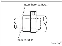
To reinstall the rubber hose securely, make sure of hose insertion length and clamp orientation. (If tube is equipped with hose stopper, insert rubber hose into tube until it butts up against hose stopper.)
