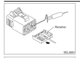
Some connectors do not have a notch above each terminal. To probe each terminal, remove the connector retainer to make contact space for probing.
