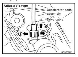
5. Loosen nuts, and remove accelerator pedal assembly.
