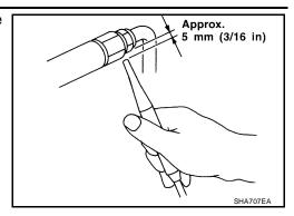
2. When checking for leaks, circle each fitting completely with the probe as shown.
