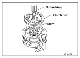
5. Install the clutch pulley bolt using Tool, to prevent the clutch disc from turning and tighten the bolt to specification. Refer to <a href="MTC-102">MTC-102</a>, "COMPONENTS"</a>.
