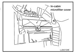
Insert the first new in-cabin microfilter into the heater and cooling unit housing and slide it over to the right. Insert the second new in-cabin microfilter into the heater and cooling unit housing.
