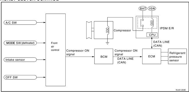
When the A/C switch is pressed, or the mode dial is turned to the defroster position, the front air control outputs a compressor ON signal to BCM.
