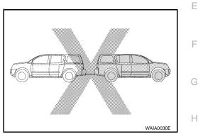
NISSAN does not recommend towing automatic transmission equipped vehicles with the drive wheels on the ground. **CAUTION:**
