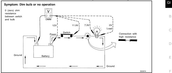
Measuring Voltage Drop — Steb-by-Step
