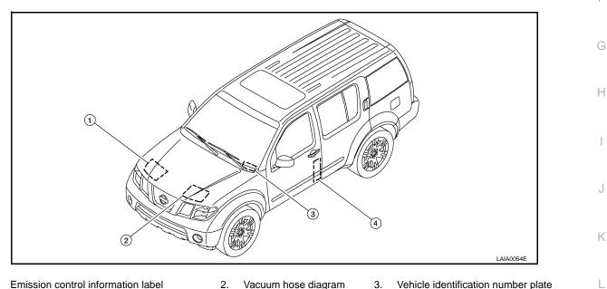
1. Emission control information label 2. Vacuum hose diagram 3. Vehicle identification number plate
