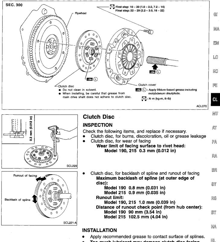
Too much lubricant may damage clutch disc facing.
