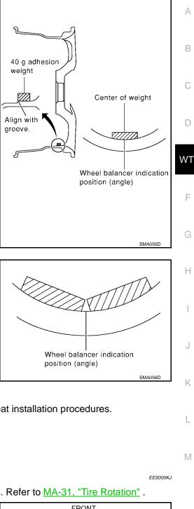
c. If calculated balance weight value exceeds 50 g (1.76 oz.), install two balance weight sheets in line with each other as shown.
