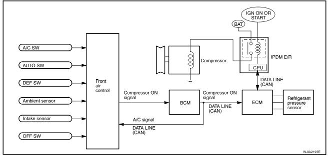
When A/C switch or DEF switch is pressed, front air control inputs compressor ON signal to BCM.
