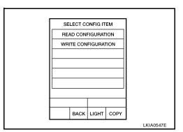
Configuration of current BCM is printed out automatically. A listing of manual setting items and auto setting items will be displayed. Auto setting items are preset and cannot be changed. Manual setting items can be set by using WRITE CONFIGURATION PROCEDURE. Refer to <a href="BCS-22">BCS-22</a>, "WRITE CONFIGURATION PROCEDURE"
