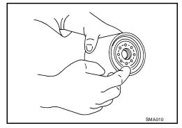
3. Screw the oil filter manually until it touches the installation surface, then tighten it by 2/3 turn. Or tighten to specification.
