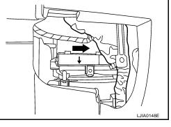
5. Install the in-cabin microfilter cover.
